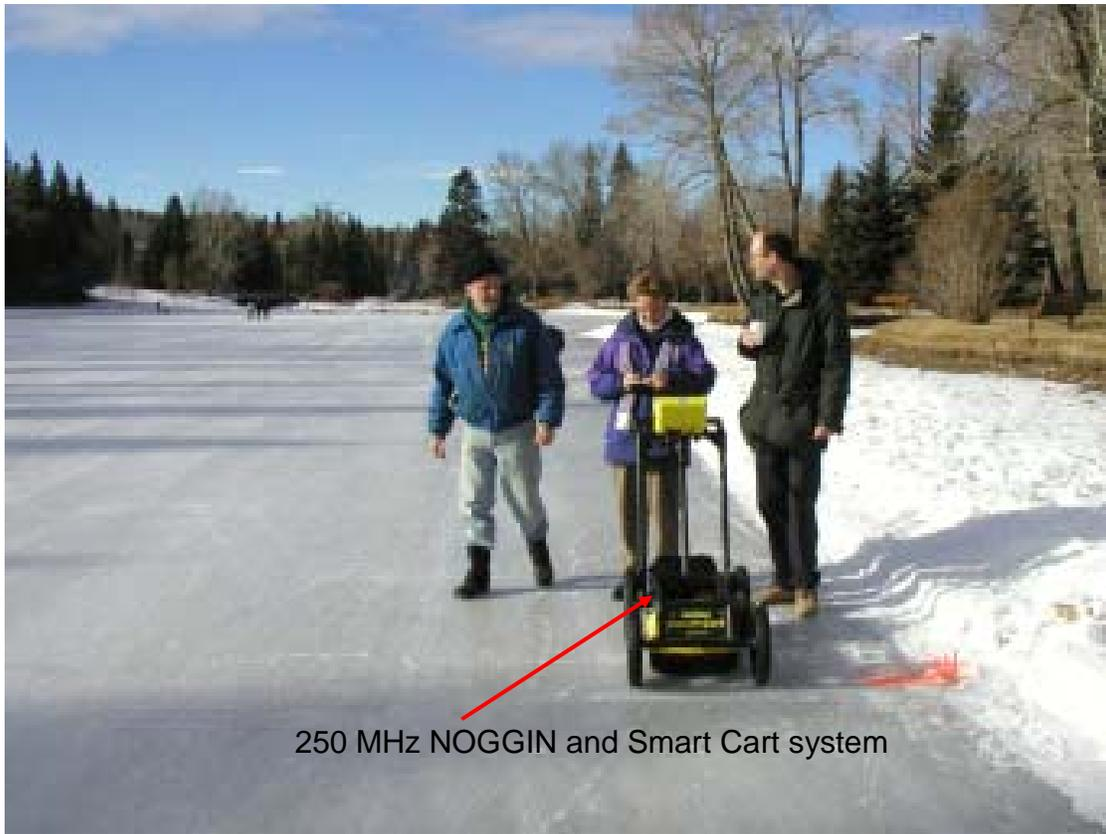
FIG. 2. Dr. Larry Bentley and Ms. Julie Aitken of the University of Calgary and Mr. Greg Johnston of Sensors and Software Ltd. conduct a GPR survey, with the Noggin® 250 MHz SmartCart®, over the frozen lagoon at Bowness Park, Calgary.
