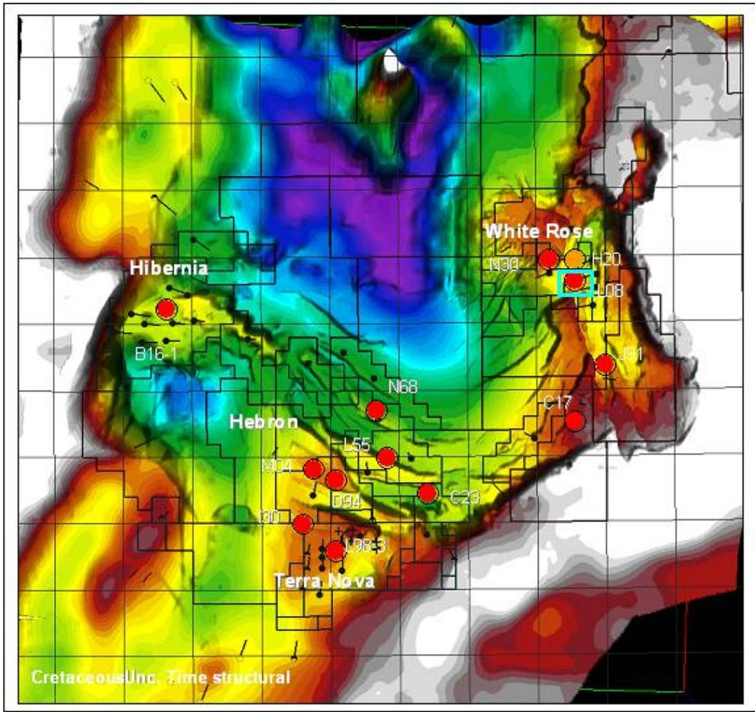
FIG. 2. Study data location – Isochron map of the Jeanne d’Arc Basin Late Cretaceous interval (white 0 ms to purple 4000 ms). Red and Orange dots are the location of individual wells in the study. The Orange dot is the location of White Rose H20 offset VSP and the Blue Square is the location of the CREWES White Rose L08 OBS survey.
