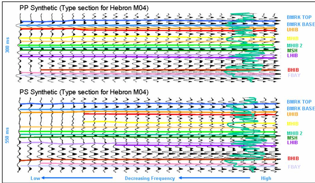
FIG. 11. Hibernia Formation PP (top) and PS (bottom) synthetic response with gamma ray log and horizon interpretation.
