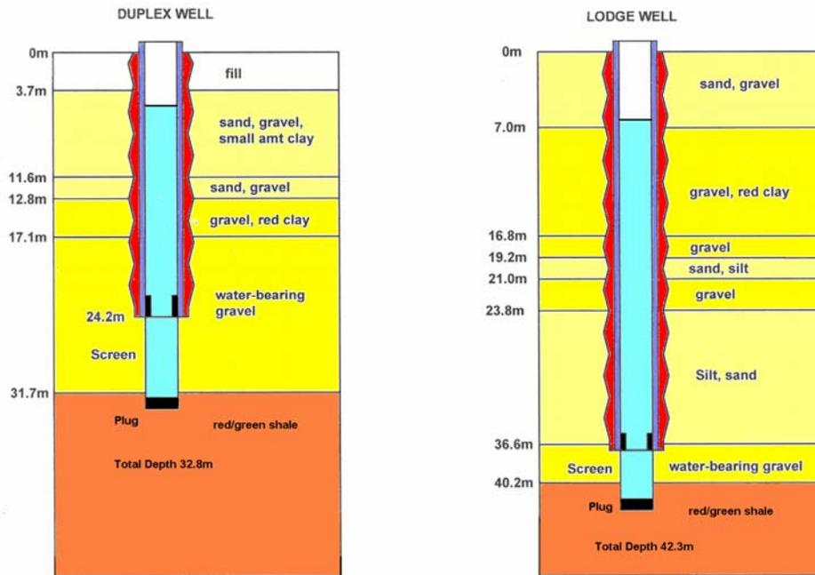
FIG. 2. Vertical section showing the construction of the Duplex and Lodge Wells. The red material around the outsides of the casings is a bentonite seal used to prevent vertical groundwater flow.
