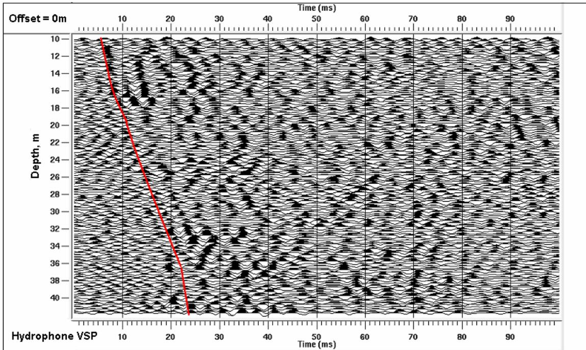
FIG. 5. Hydrophone VSP with source offset of 0 m. Apparent velocities are about 1600 m/s to 1750 m/s; however, the time picks are not reliable.
