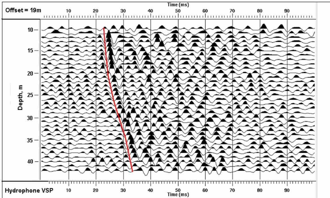
FIG. 7. Hydrophone VSP with source offset of 19 m. Calculated velocities are about 1000 m/s to 1300 m/s, depending on how the arrival times are picked.
