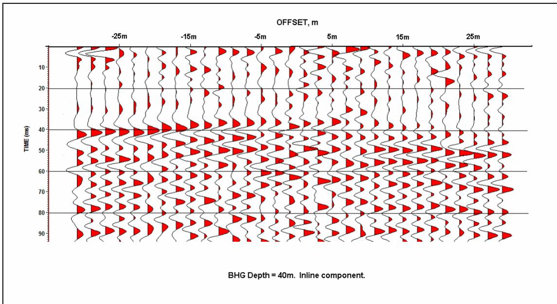
FIG. 14. Walk-away profile (inline component) with geophone depth of 40 m. Traces are plotted with AGC emphasizing the early P-wave arrival.
