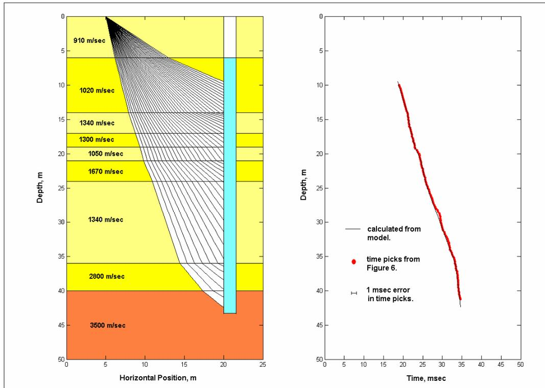
FIG. 15. Ray-tracing and fitting of first arrival times picked from the 15m offset VSP of Figure 6 using a layered velocity model. Left: The model with a sample of refracted rays. Right: Comparison of the observed times with the calculated times from the ray tracer.
