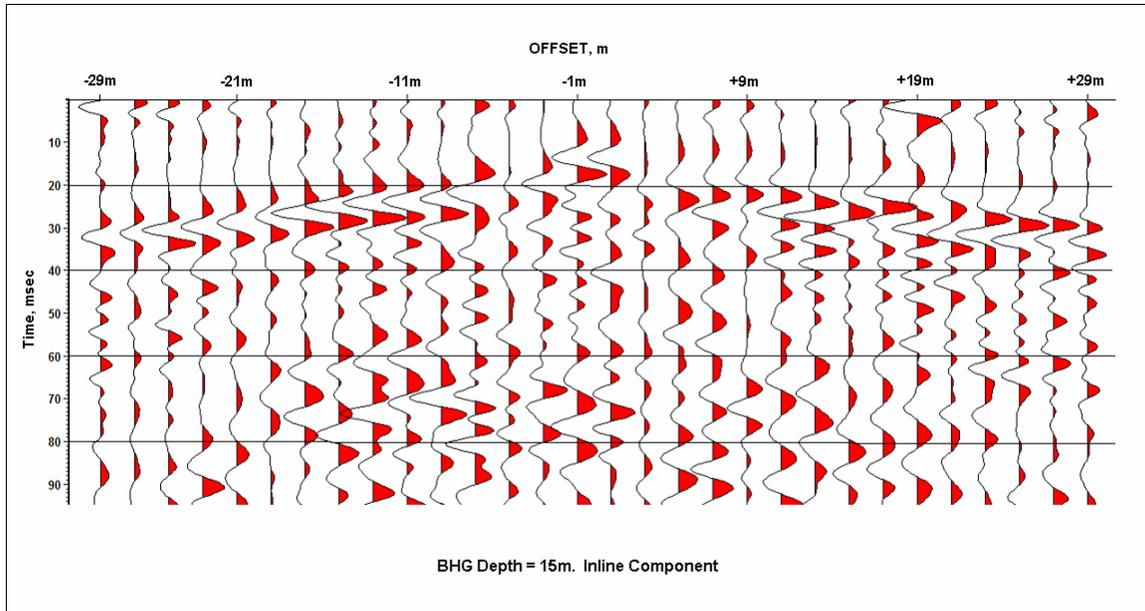
FIG. 13. Walk-away profile (inline component) with geophone depth of 15m. Traces are plotted with AGC emphasizing the early P-wave arrival.
