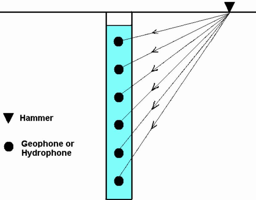
FIG. 3. Depth profile shooting with fixed source offset.
