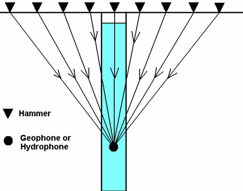
FIG. 4. Source walk-away profile with fixed downhole detector.
