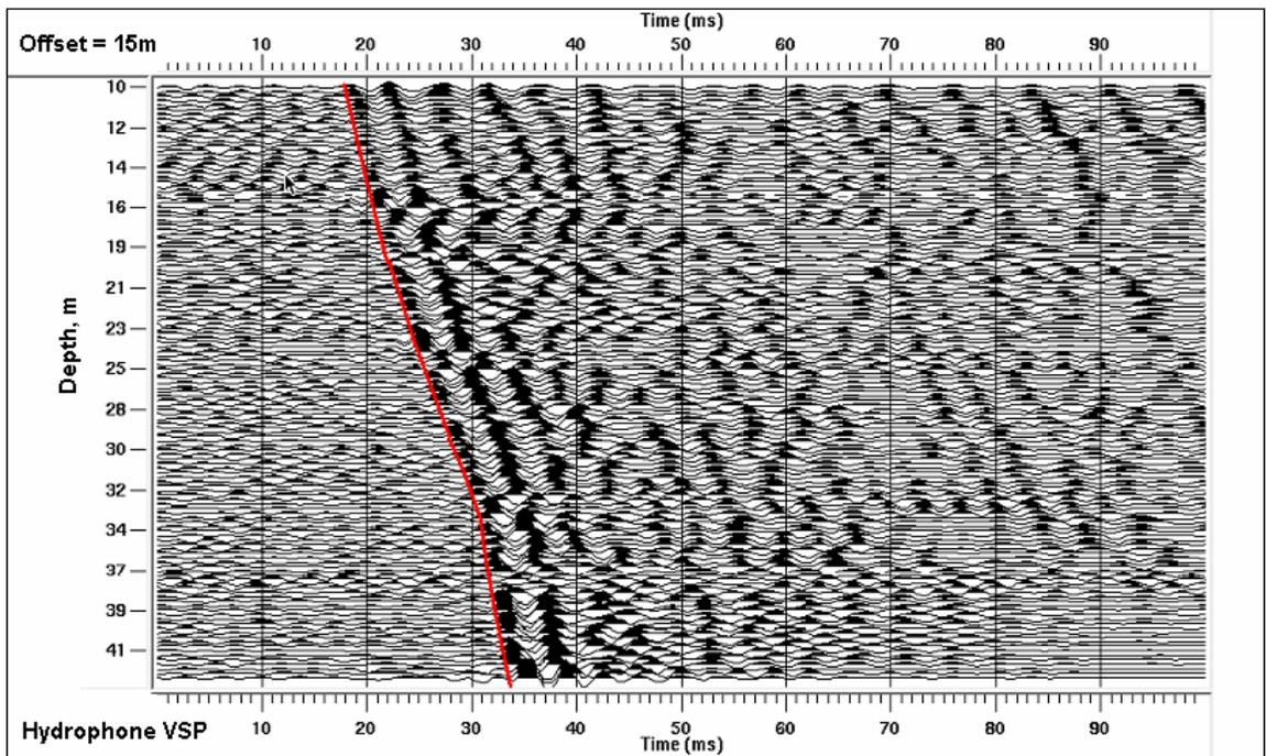
FIG. 6. Hydrophone VSP with source offset of 15m. Calculated apparent velocities are in the range 1050 m/s to 1310 m/s.
