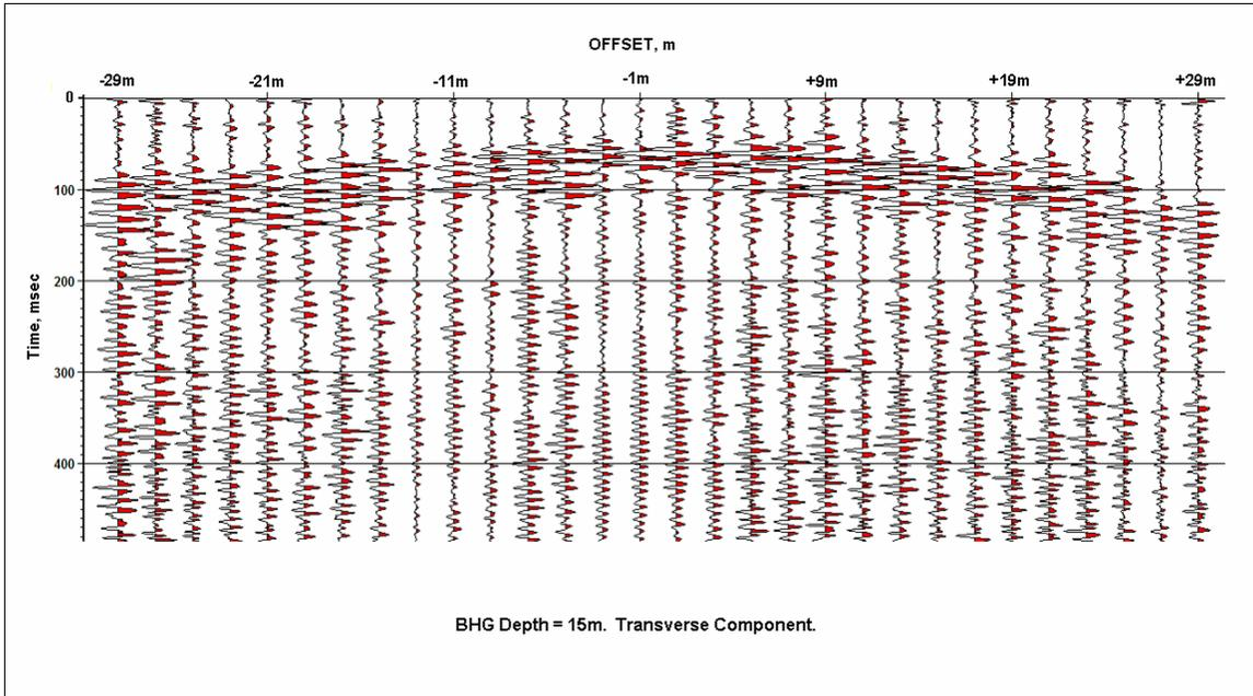
FIG. 11. Walk-away gather (transverse component) with geophone depth of 15 m. Traces are plotted with AGC emphasizing the S-wave arrival.
