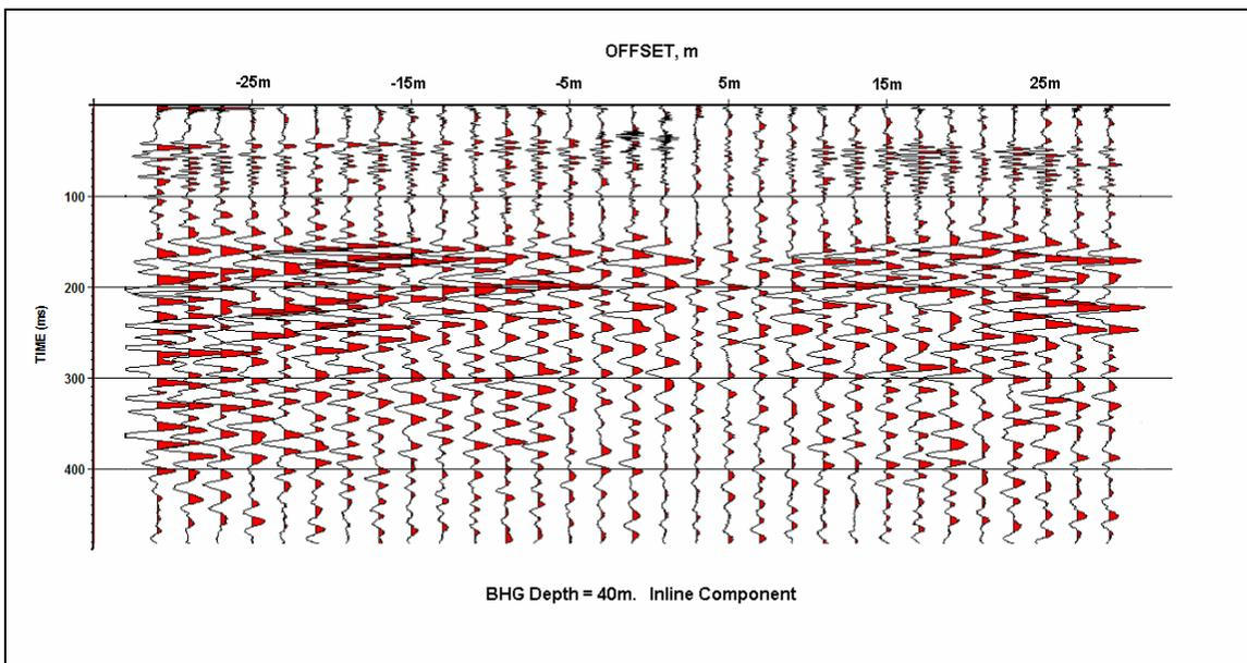
FIG. 12. Walk-away profile (inline component) with geophone depth of 40m. Traces are plotted with AGC emphasizing the S-wave arrival.
