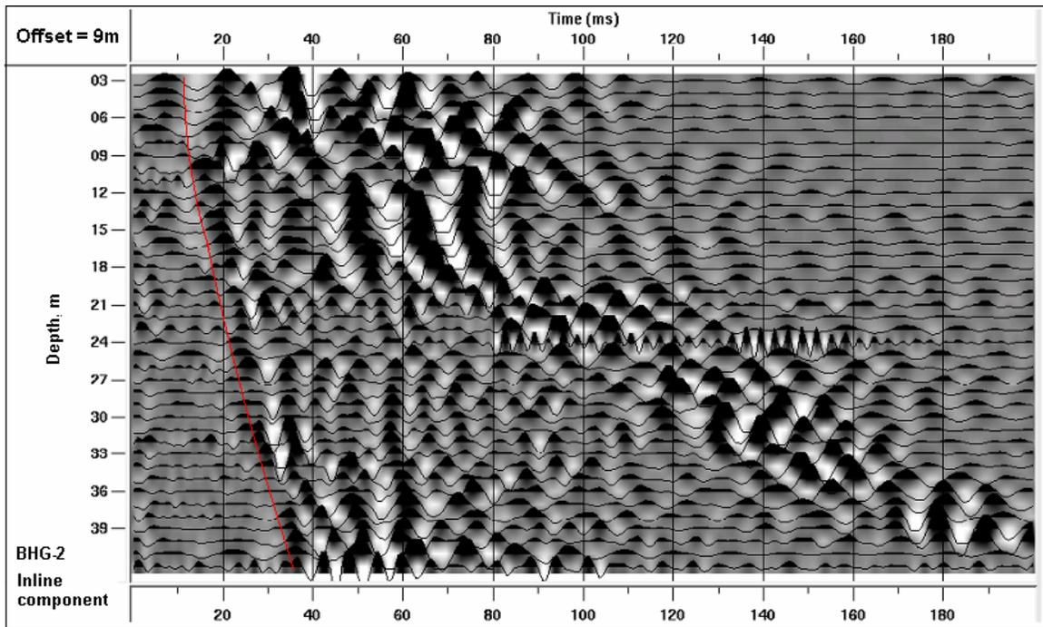
FIG. 9. Geophone-recorded VSP (inline component) with source offset of 9m.
