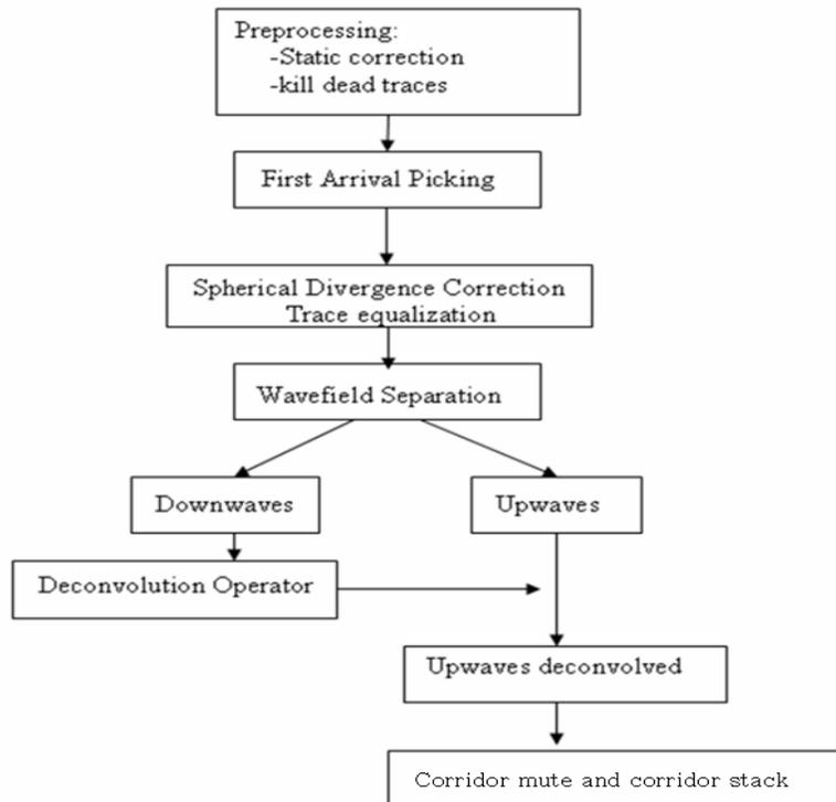
FIG. 4. Processing flow for zero-offset VSP data (Hinds and Kuzmiski, 2006).
