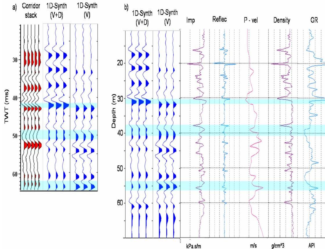
FIG. 8. a) VSP corridor stack (left) and 1-D synthetic seismograms indexed in their two-way-travel time, b) Correlation of 1-D synthetic seismogram with the well logs in their depths.
