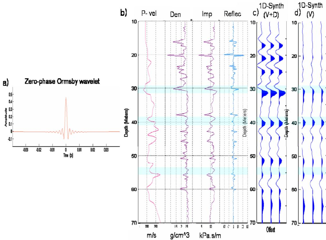
FIG. 7. a) Zero-phase Ormsby wavelet using the frequency bandwidth of [5 15 450 500] Hz (see Figure 6a), b) Impedance and reflectivity were computed based on the density and sonic log, c) 1-D synthetic seismogram generated by convolving the wavelet (a) with the reflectivity (b), d) 1-D synthetic seismogram generated using the sonic log and estimated density function. Y-axis of all logs and seismograms are indexed in depth.
