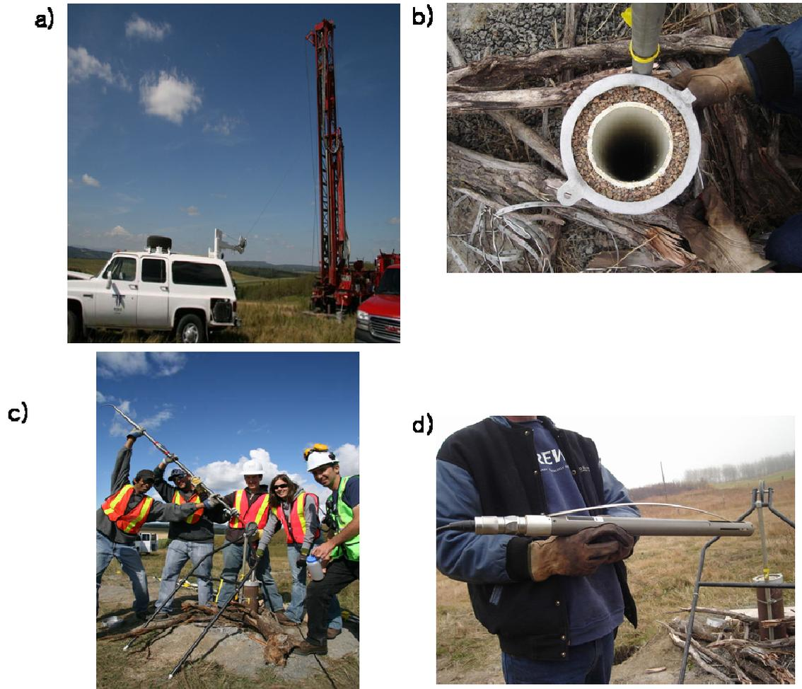
FIG. 1. a) 4.5 inch inner-diameter of the test well, b) Roke Well logging company's logging unit, c) deploying full-waveform sonic log tool, d) clamping-geophone used for VSP survey.
