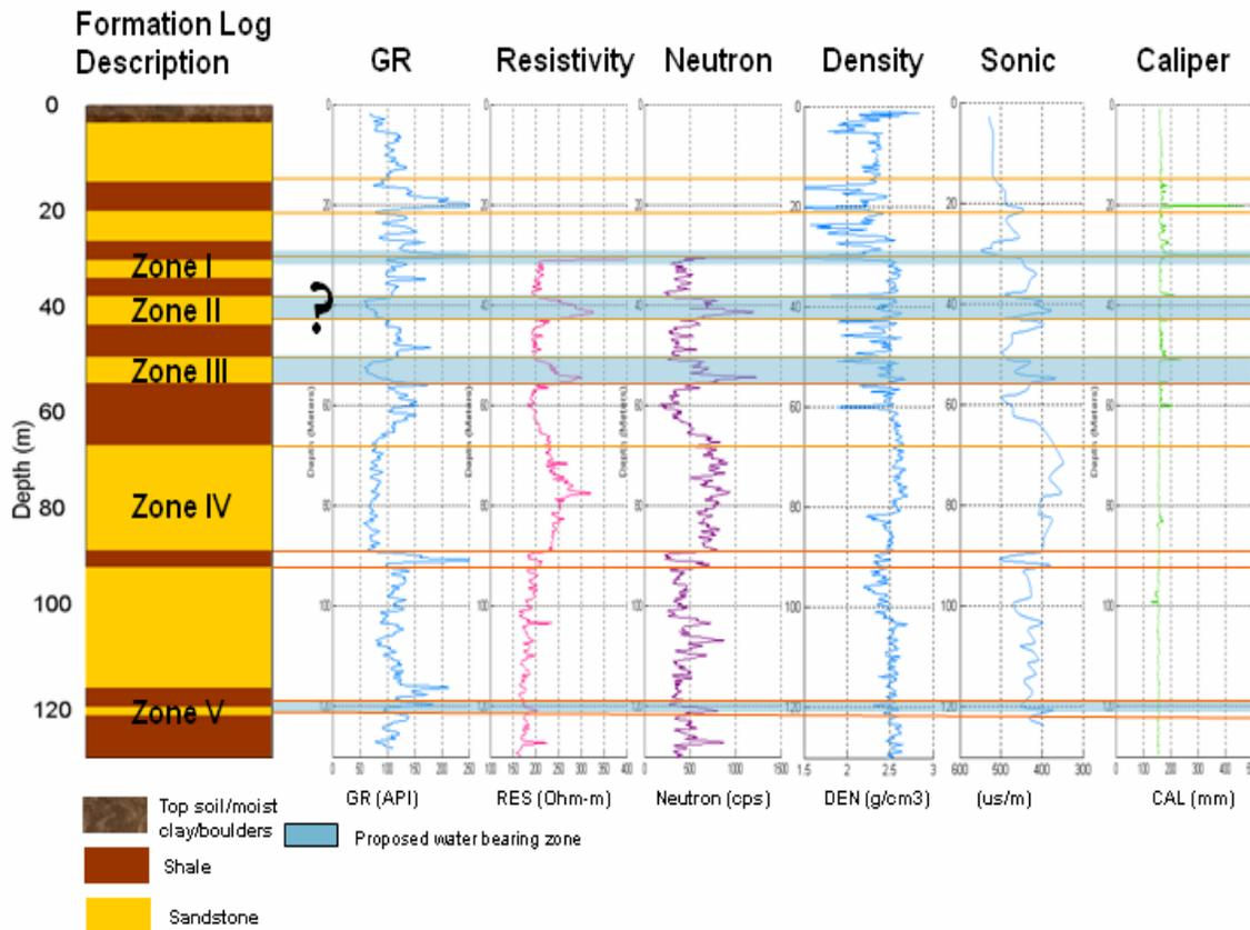
FIG. 2. Formation log description recorded insitu while drilling (far left) and well logs acquired from Priddis test well.
