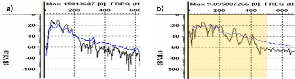
FIG. 5. a) Up-going wavefields before deconvolution, b) Up-going wavefields after deconvolution; the yellow box indicates the frequency bandwidth used to generate a zero-phase ormsby wavelet used for 1-D synthetic seismogram.
