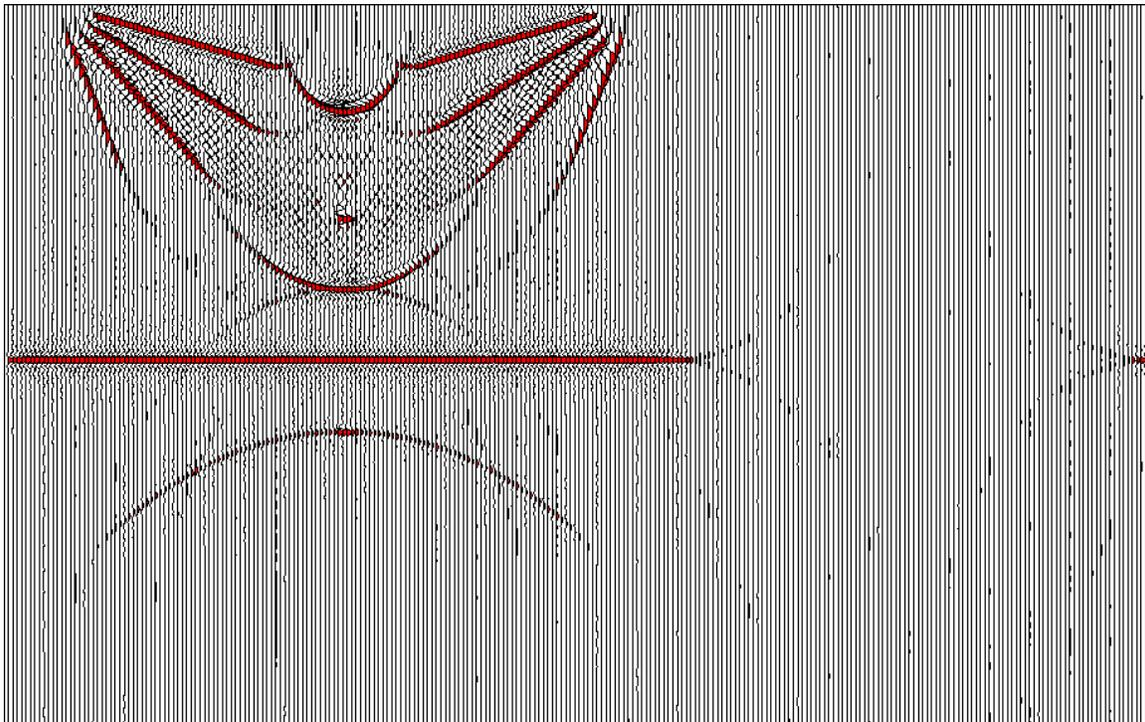
FIG. 4. Migrated section resulting from the linear interpolation method. Downturned curves connected to the spikes and the upturned semi-circles, and weak curves at the ends of the terminating reflectors are artifacts.
