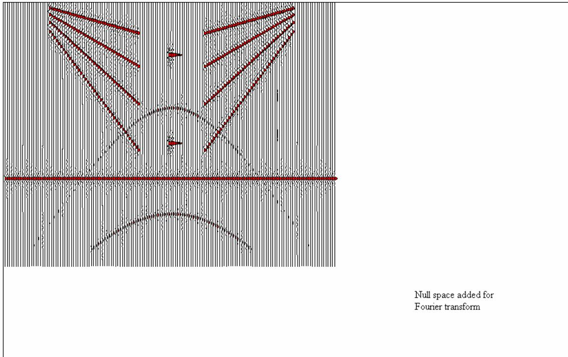
FIG. 1. Model of stacked section. It has a seismic data set of 150 traces and 750 samples in each trace. However, it is shown as 256 traces and 1024 samples in each trace for the sake of comparison with the migrated sections, which have 256 traces and 1024 samples in each trace.
