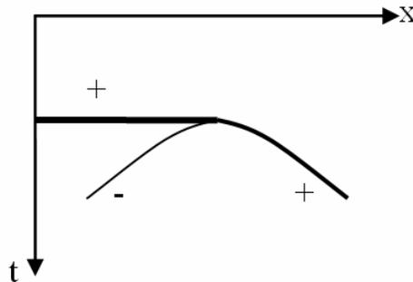
FIG. 2. A terminating reflector in a CMP stack section should show diffractions. The reflector and the forward branch have the same pulse polarity, the backward branch have the opposite pulse polarity. (Adapted from Krebs, 2006)
