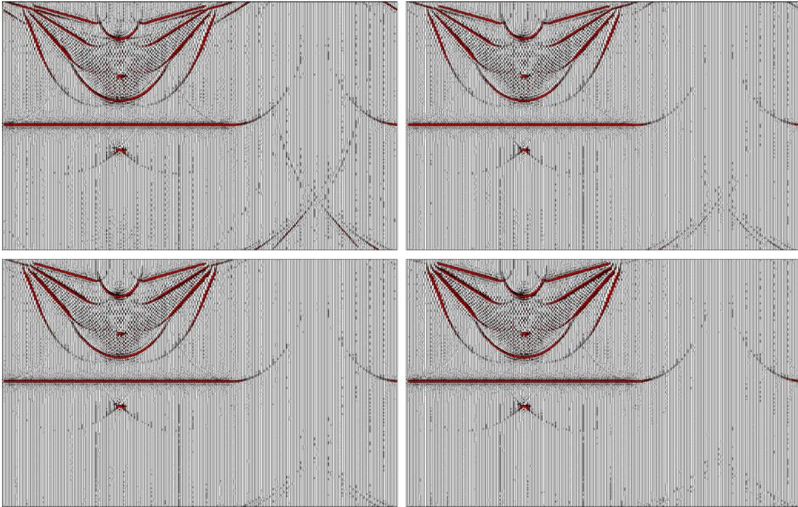
FIG. 7. Migrated sections resulted from complex sinc interpolation method. These are the results of using two (top-left), four (top-right), eight (bottom-left) and sixteen (bottom-right) samples in line to interpolate. Artifacts are gradually attenuated when the number of samples used in interpolation increases.
