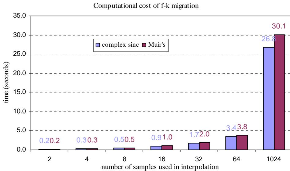
FIG. 10. Computational costs of f-k migration using complex sinc interpolation and Muir's interpolation. The costs of the two interpolation methods are comparable.
