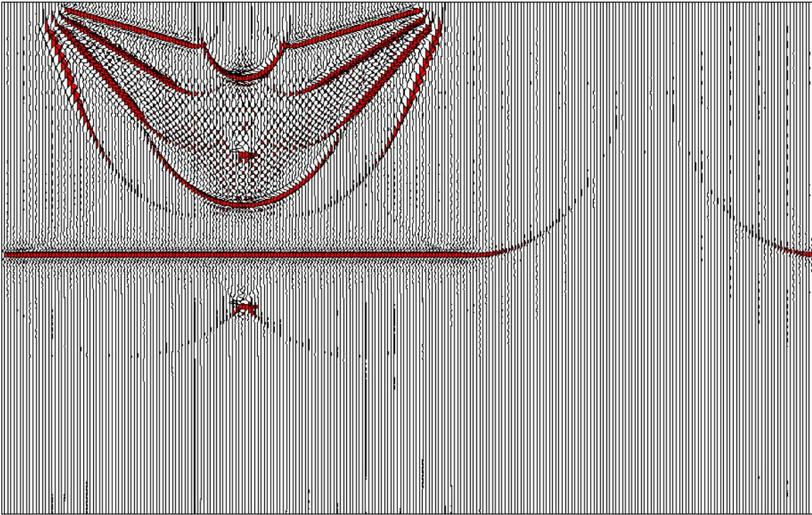
FIG. 6. Migrated section resulted from complex sinc interpolation method. This is the result of using all the 1024 samples in line to interpolate. Artifacts are significantly attenuated.
