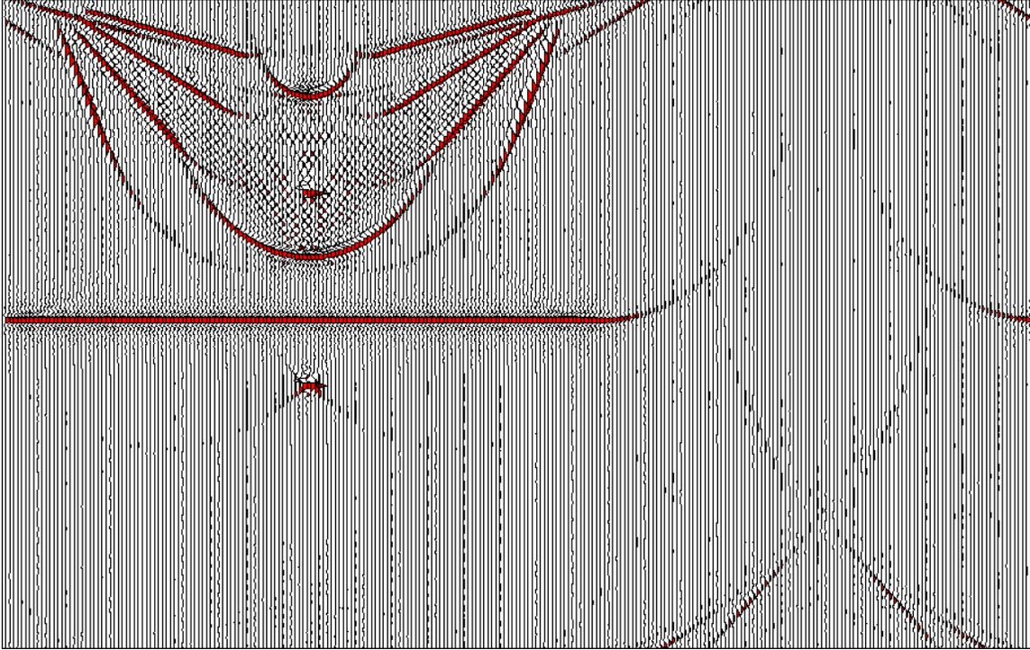
FIG. 5. Migrated section resulted from complex linear interpolation method. The dark lines parallel to the dips are artifacts.
