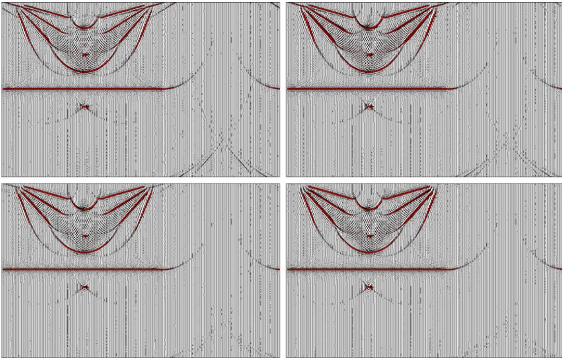
FIG. 9. Migrated sections resulted from Muir's interpolation method. These are the results of using two (top-left), four (top-right), eight (bottom-left) and sixteen (bottom-right) samples in line to interpolate. The results are similar to those of complex sinc interpolation.
