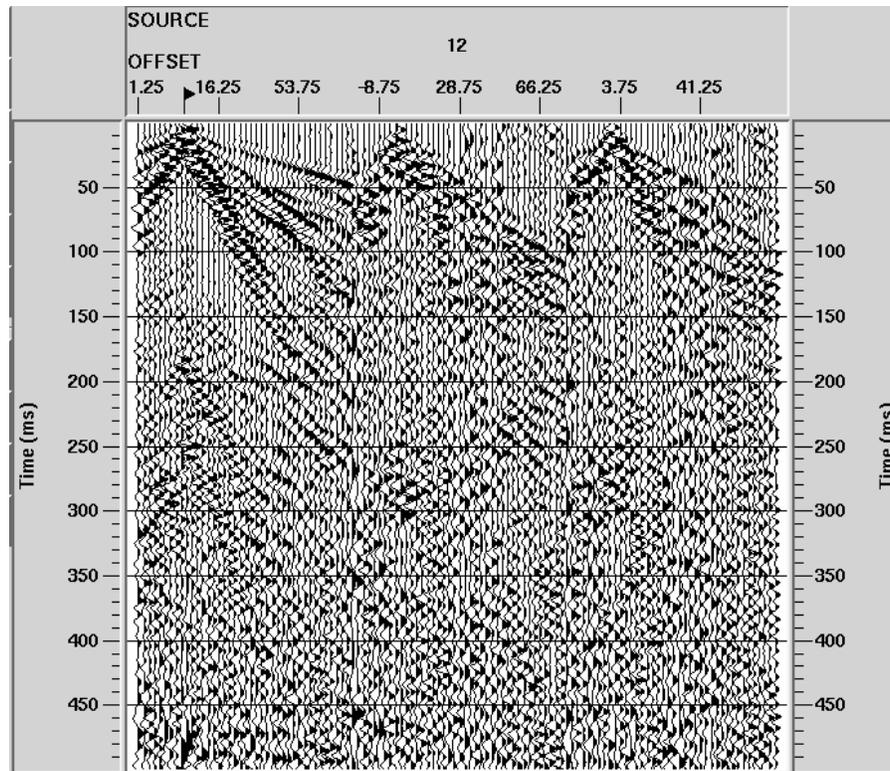
FIG. 6. Three-component shot gather for Area 4: vertical component (left), transverse component (middle) and radial component (right).
