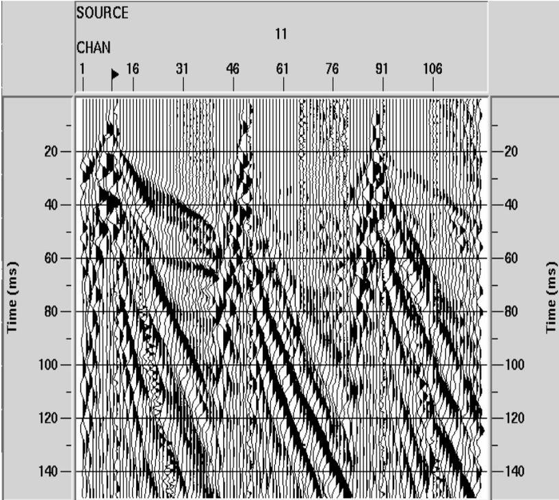
FIG. 5. Three-component shot gather for Area 3: vertical component (left), transverse component (middle) and radial component (right).
