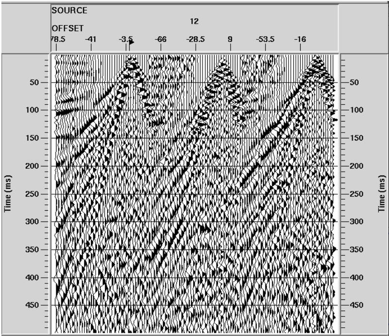
FIG. 4. Three-component shot gather for Area 1: vertical component (left), transverse component (middle) and radial component (right).
