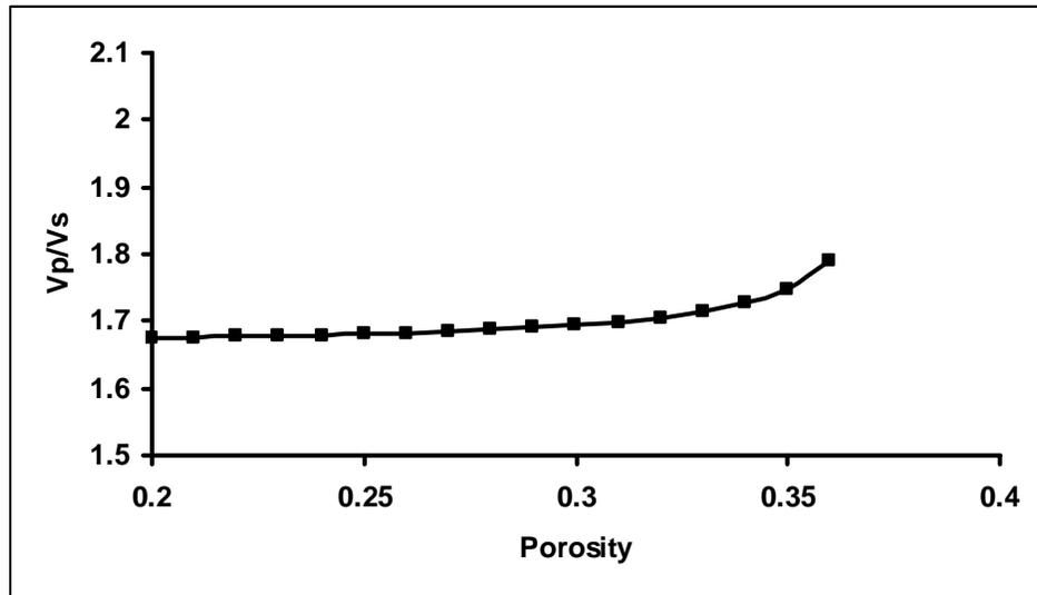
FIG. 2. The effect of porosity on  $V_p/V_s$  ratio.
