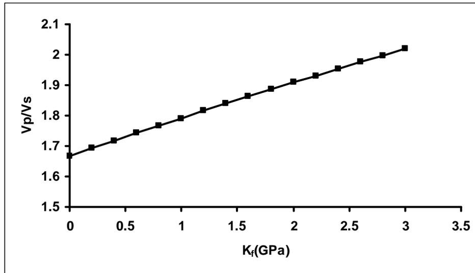
FIG. 1. The effect of  $K_f$  on  $V_p/V_s$  ratio.
