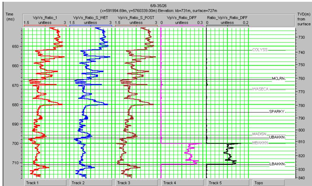
FIG. 3. All three  $V_p/V_s$  ratios for pre-production, wet and post-production conditions after fluid substitution and the difference of  $V_p/V_s$  ratios between post- and pre-production conditions.
