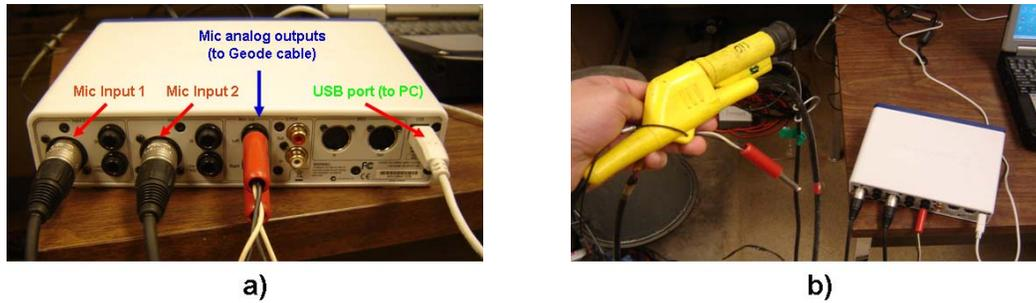
FIG. 4. Two studio microphones were connected to the analog inputs of a Digidesign MBox2 (left) using conventional microphone XLR cables. The MBox2 analog outputs were connected to the Geode receiver cable through special cables consisting of jack connectors on one end and single-pin geophone connectors on the other (right).
