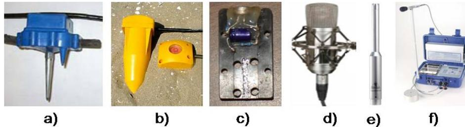
FIG. 2. Seven sensors were used in the test: a) OyoGeospace GS-3C geophone, b) Input/Output Spike 3C geophone, c) CREWES microphone prototype, d) APEX 435 condenser microphone, e) EMC8000 electret-condenser microphone, and f) Blastmate III unit with two calibrated sensors (3C geophone and microphone).
