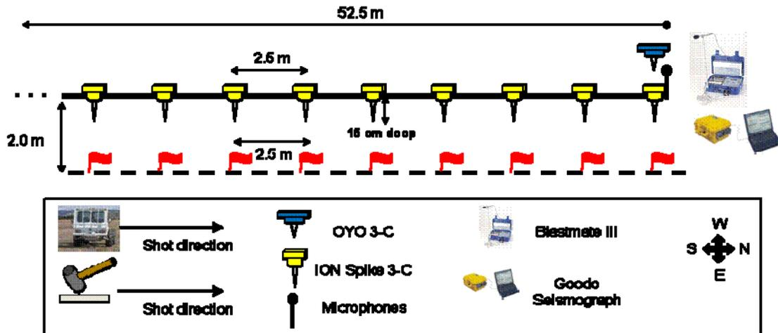
FIG. 5. Acquisition layout for shot and receiver lines.
