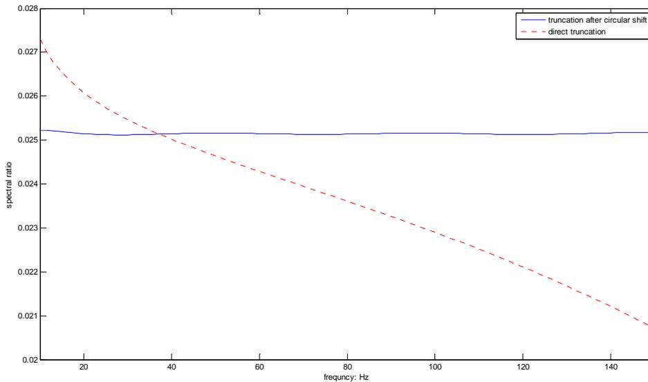
FIG. 2. Slope of amplitude (log) spectral ratio of attenuated impulse response.
