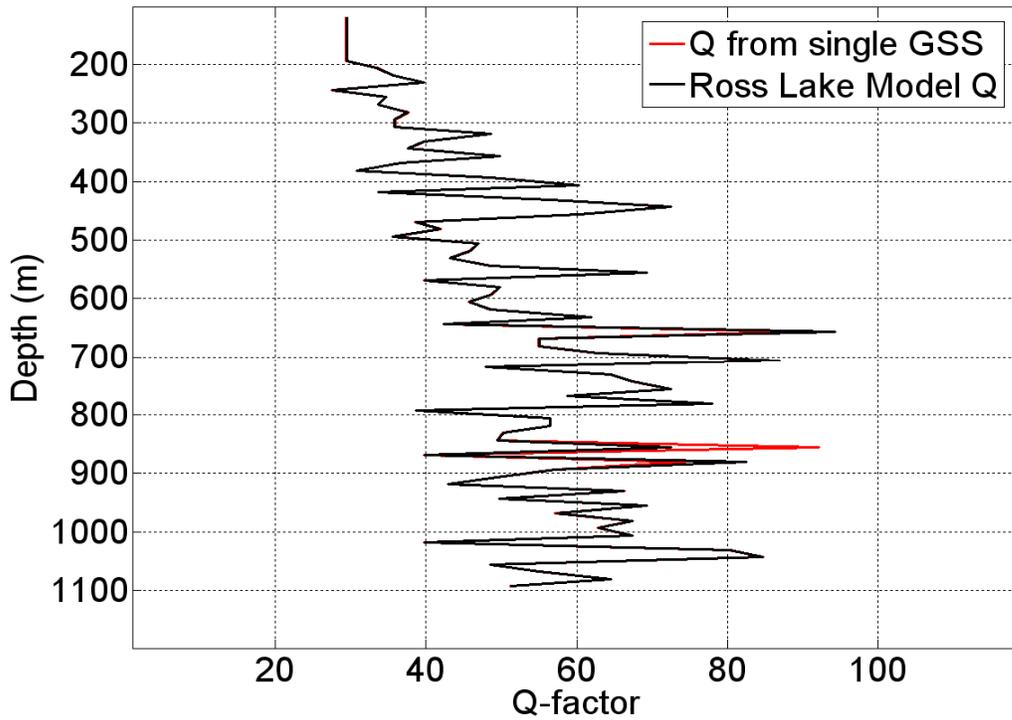
FIG.4. Q versus depth from Golden Section Search compared to Ross Lake model Q.
