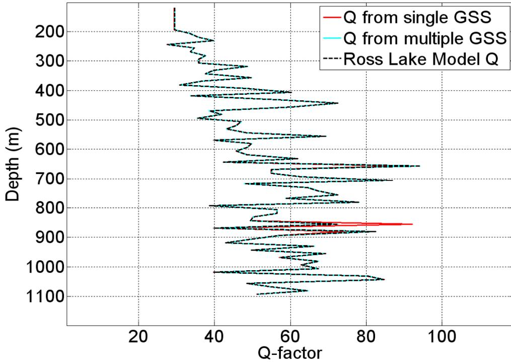
FIG.6. Q versus depth from augmented Golden Section Search compared to Figure 4.
