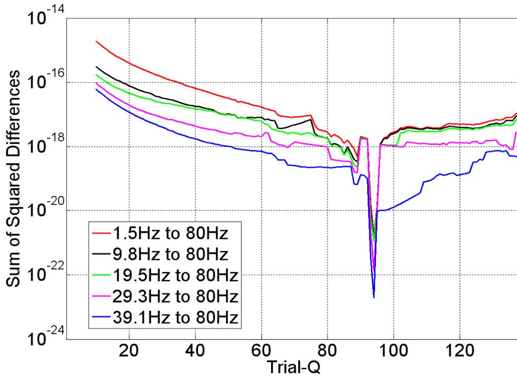
FIG.8. Bandwidth dependence of *sums-of-squared-differences* at Z=656m (Q=94.3).
