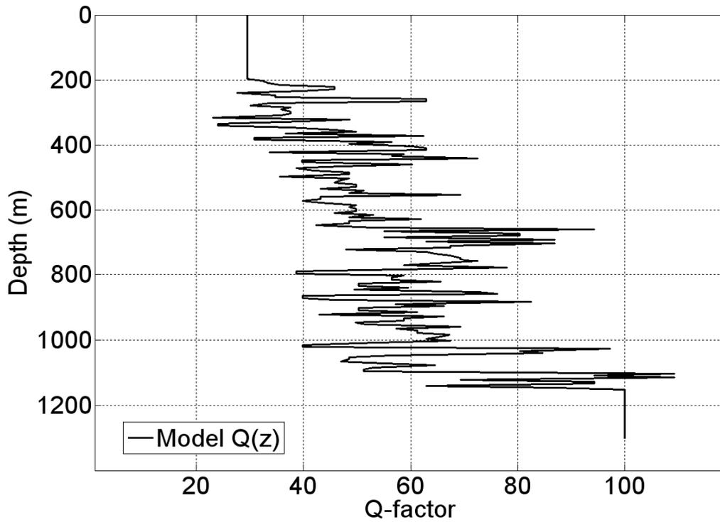
FIG.2. Q-model generated from Ross Lake P-wave velocities using Waters's equation.
