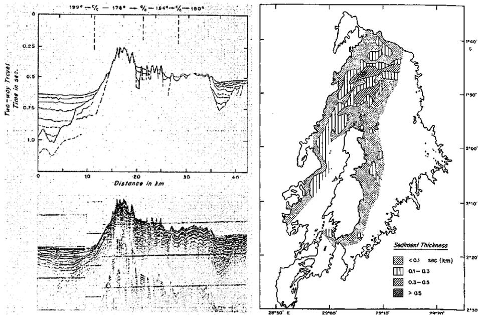
FIG. 7. An example seismic section (lower left) from seismic data acquired in 1971 (WHOI, 1971) and its interpretation (upper left) from western Lake Kivu. The resultant interpretation of sediment thickness over the survey area is displayed on the right.
