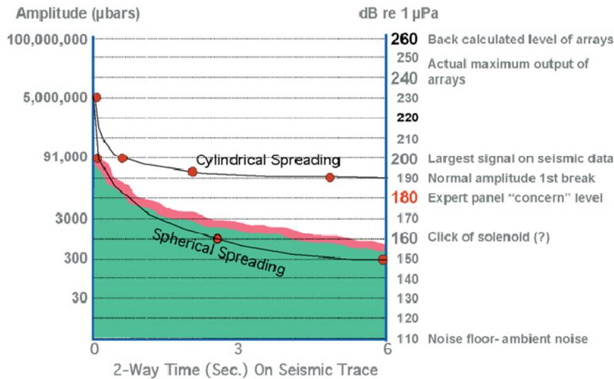
FIG. 15. Decrease of seismic energy from an airgun array as a function of two-way seismic travelttime (from Caldwell and Dragoset, 2000). Three seconds, on the horizontal axis, is equivalent to about 4500 m travel path.
