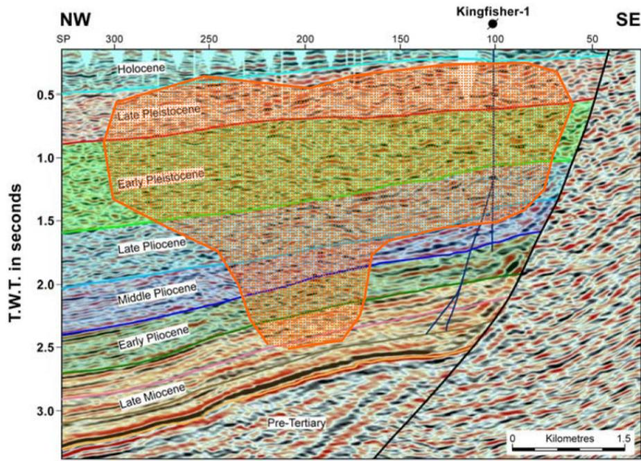
FIG. 4. Seismic line through the Kingfisher oilfield discovery with sediment ages annotated. Note the interpreted gas cloud, outlined in orange, above the reservoir (Logan et al., 2009).
