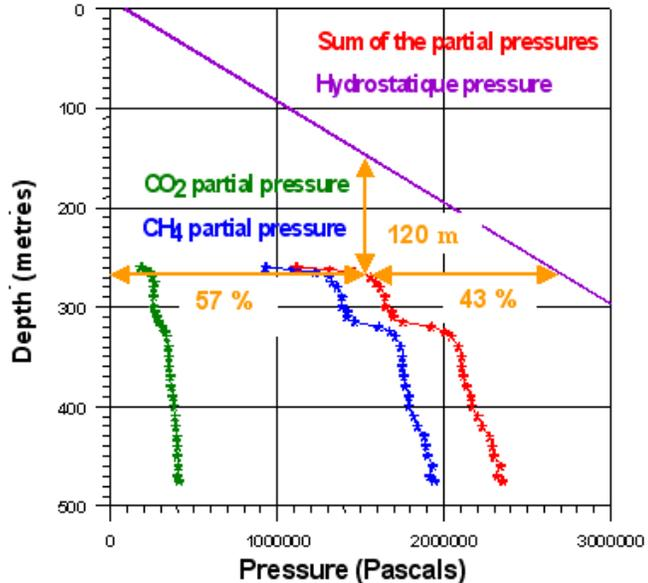
FIG. 9. Water sampling on Lake Kivu near the methane extraction facility (R. Stewart photo; January, 2010). Measurement of the gas partial pressures, total gas pressure, and hydrostatic pressure in Lake Kivu.
