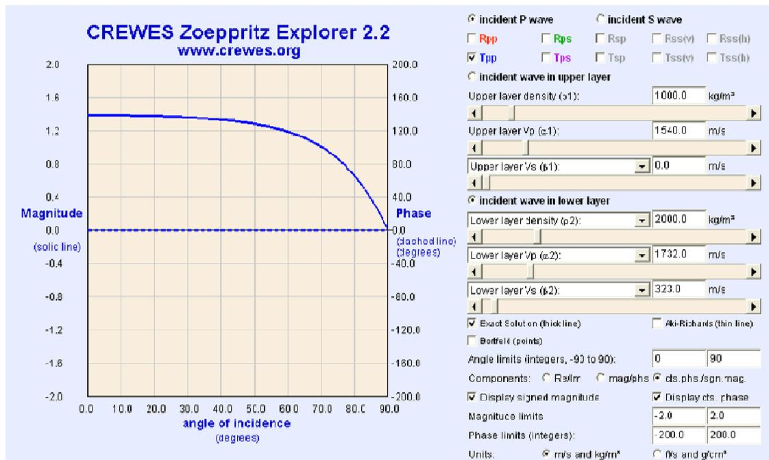
FIG. 12. A plot of the motion transmitted across a solid interface to overlying water. The upper layer is lake water while the lower layer is an estimate of the sediment properties. The CREWES (University of Calgary, Canada) motion simulator is used for the calculation.
