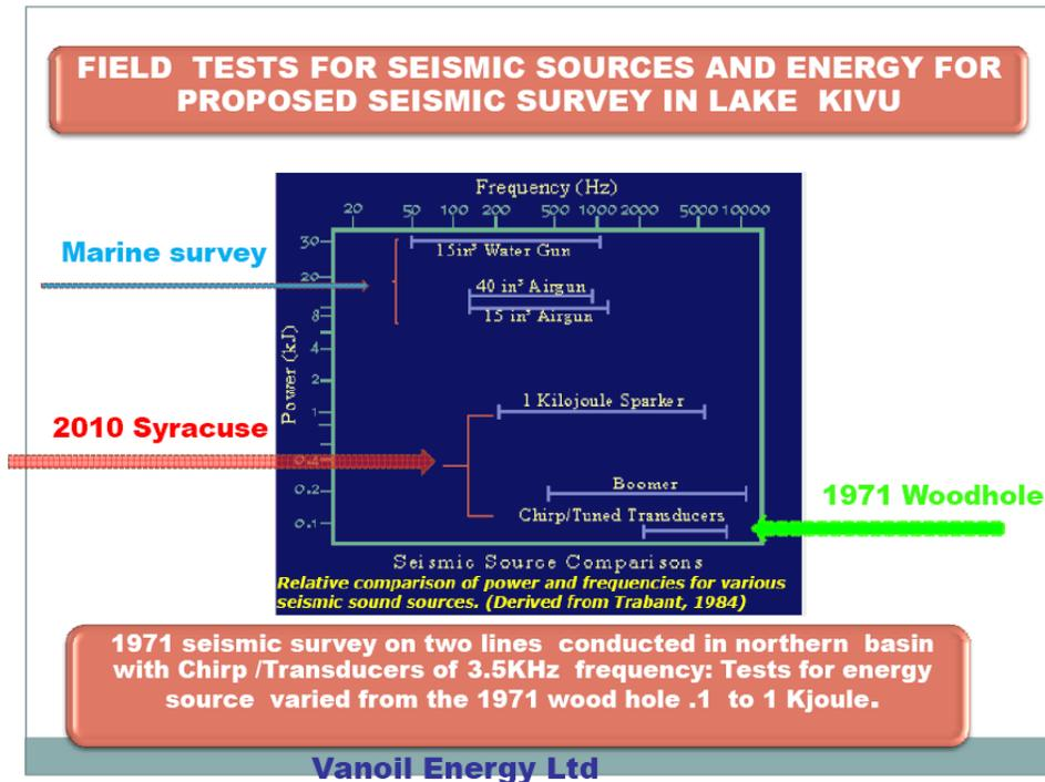
FIG. 16. Frequency range and power output of various small marine seismic sources (After Woods Hole Science Center, <http://woodhole.er.usgs.gov/operations/sfmapping/seismic.htm>).
