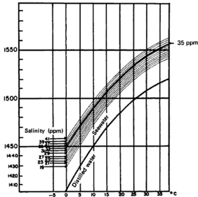
FIG. III.2.2. – Speed of sound in water (on the surface) in terms of temperature and salinity (according to Del Grosso).
