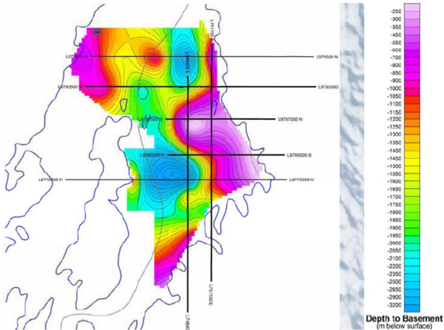
FIG. 6. Depth to the basement around northeastern Lake Kivu. Note that interpreted depths exceed 3000m (PGW, 2008).
