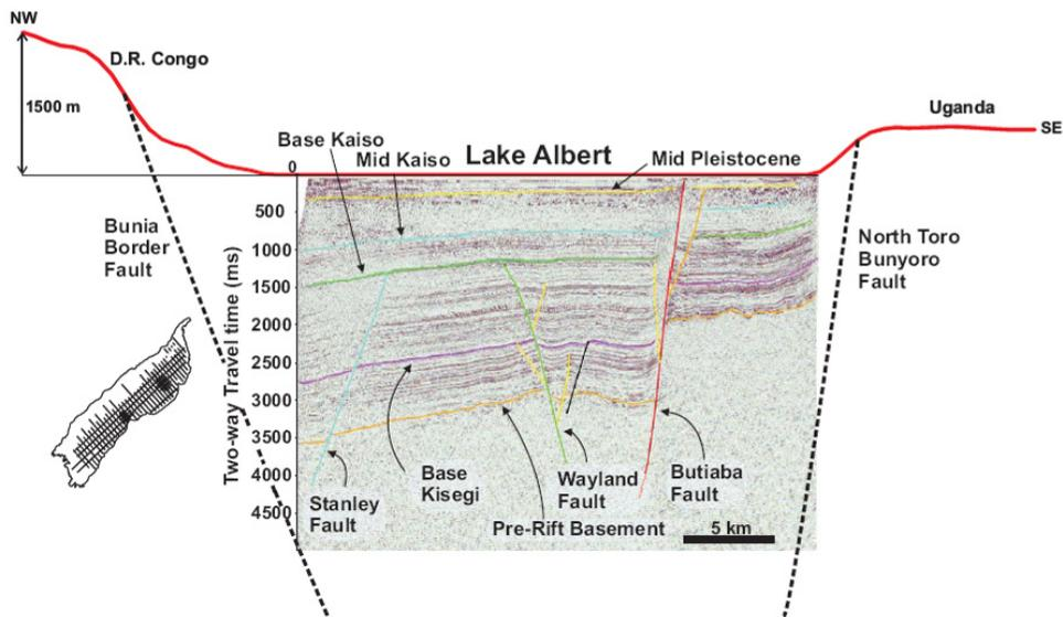
FIG. 5. Seismic section across Lake Albert, Uganda (from , 2010) indicating over 4000m (approximately corresponding to 4000ms of seismic traveltime) of sediments.
