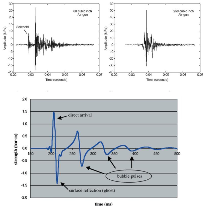
FIG. 16. Signature of marine seismic sources (above left and right) at 10 m from the source from [http://www.iwcoffice.org/\\_documents/sci\\_com/SC58docs/SC-58-E30.pdf](http://www.iwcoffice.org/_documents/sci_com/SC58docs/SC-58-E30.pdf) and a 40 cu. in. air gun signature measured at 300 m (above center) from Dragoset (2000).
