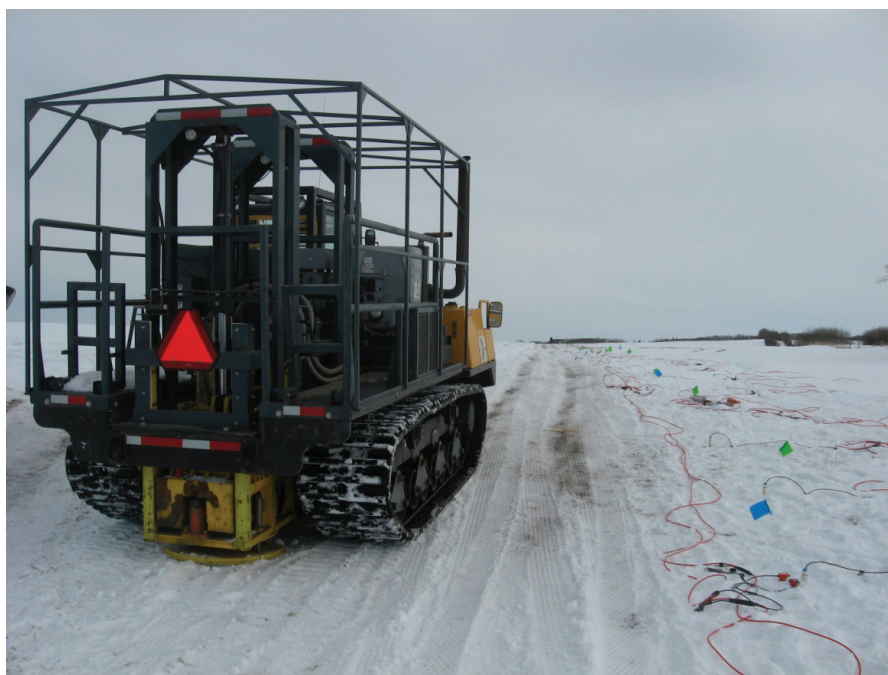
FIG. 3. The rear of the onSEIS vehicle with the source resting on the ground ready for a shot.
