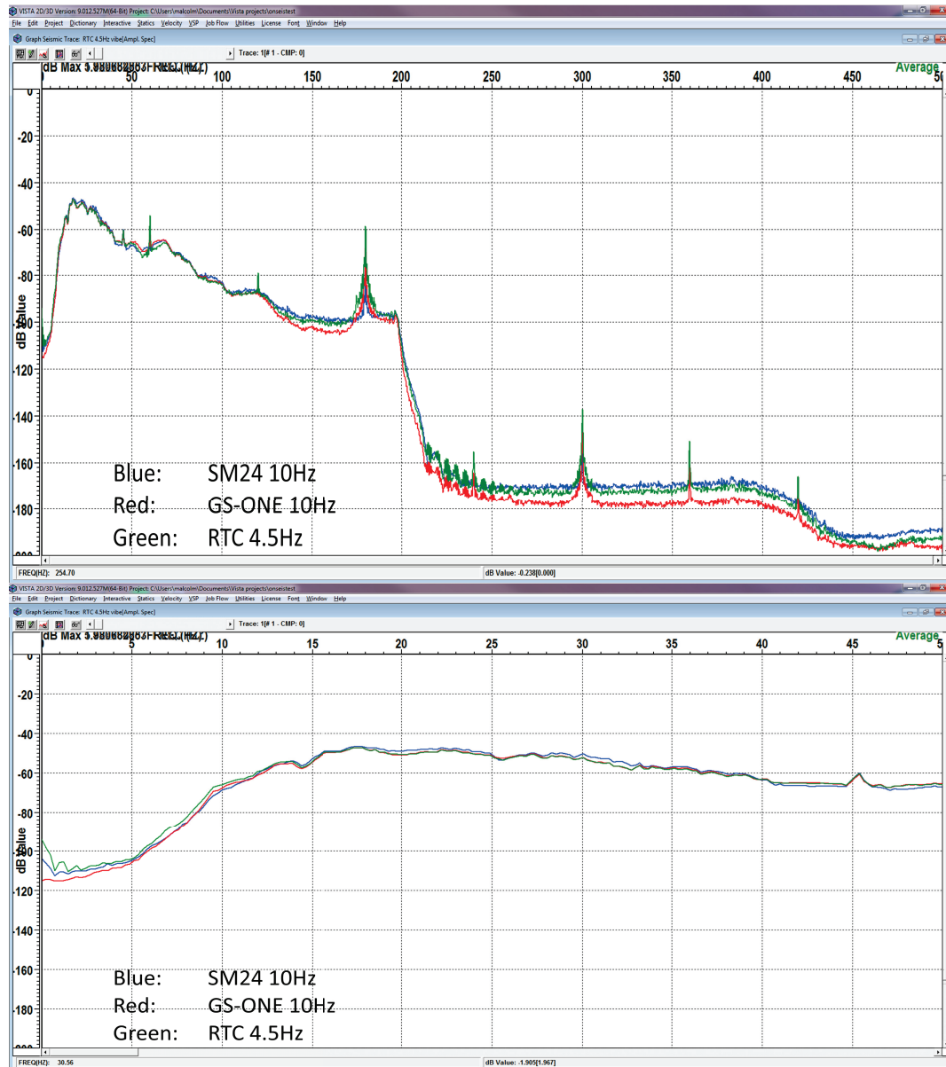
FIG. 25. The spectra for the receiver gathers at flag 109 for vibe shots from flag 112 to 180.
