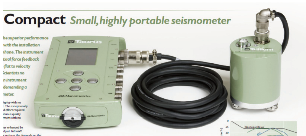
FIG. 1. Nanometrics Taurus recorder and Trillium compact seismometer (Nanometrics, 2011).
