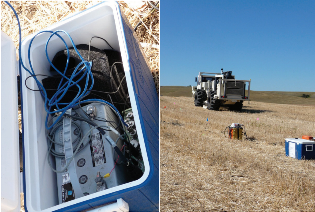
FIG. 2. Car battery and Taurus recorder inside a food cooler (left), and on the ground near VectorSeis and Aries equipment, during an INOVA 364 low-frequency vibe sweep (right).
