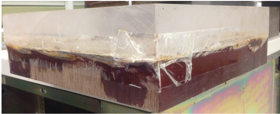
FIG. 1. A physical model consisting of a Phenolic layer under a Plexiglas layer, and representing a fractured reservoir overlaid by isotropic overburden. Laboratory to field scale is 1:10,000 in both length and time. Scaled thicknesses of Plexiglas and Phenolic layers are 480 m and 450 m respectively.
