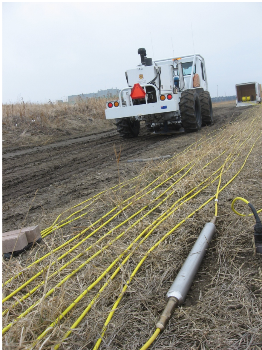
FIG. 18. The vibe being used as a source for the equipment test.
