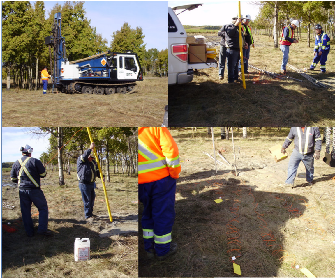
FIG. 26. Drilling and loading the multi-depth charges for the up hole experiment, note the number of shot leads in the bottom right.
