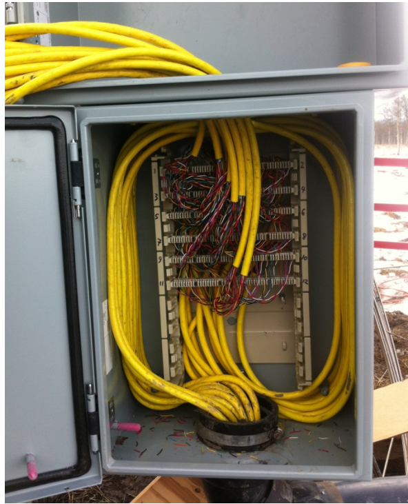
FIG. 30. Reorganizing the cemented downhole geophones while at the same time reducing the cable length to something more manageable.
