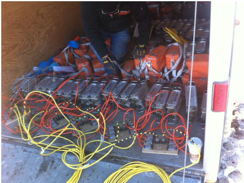
FIG. 31. Connecting newly shortened cables to the Aries system through the adapter boards.
