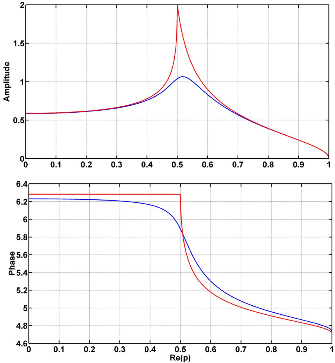
Fig. 11. The  $R_{12}^{SH}$  transmission coefficient at an interface between two anelastic media. The upper (1) medium has  $Q_1 = 20$  while in the lower (2) medium  $Q_2 = 5$ . Medium parameters are given in Table 2.
