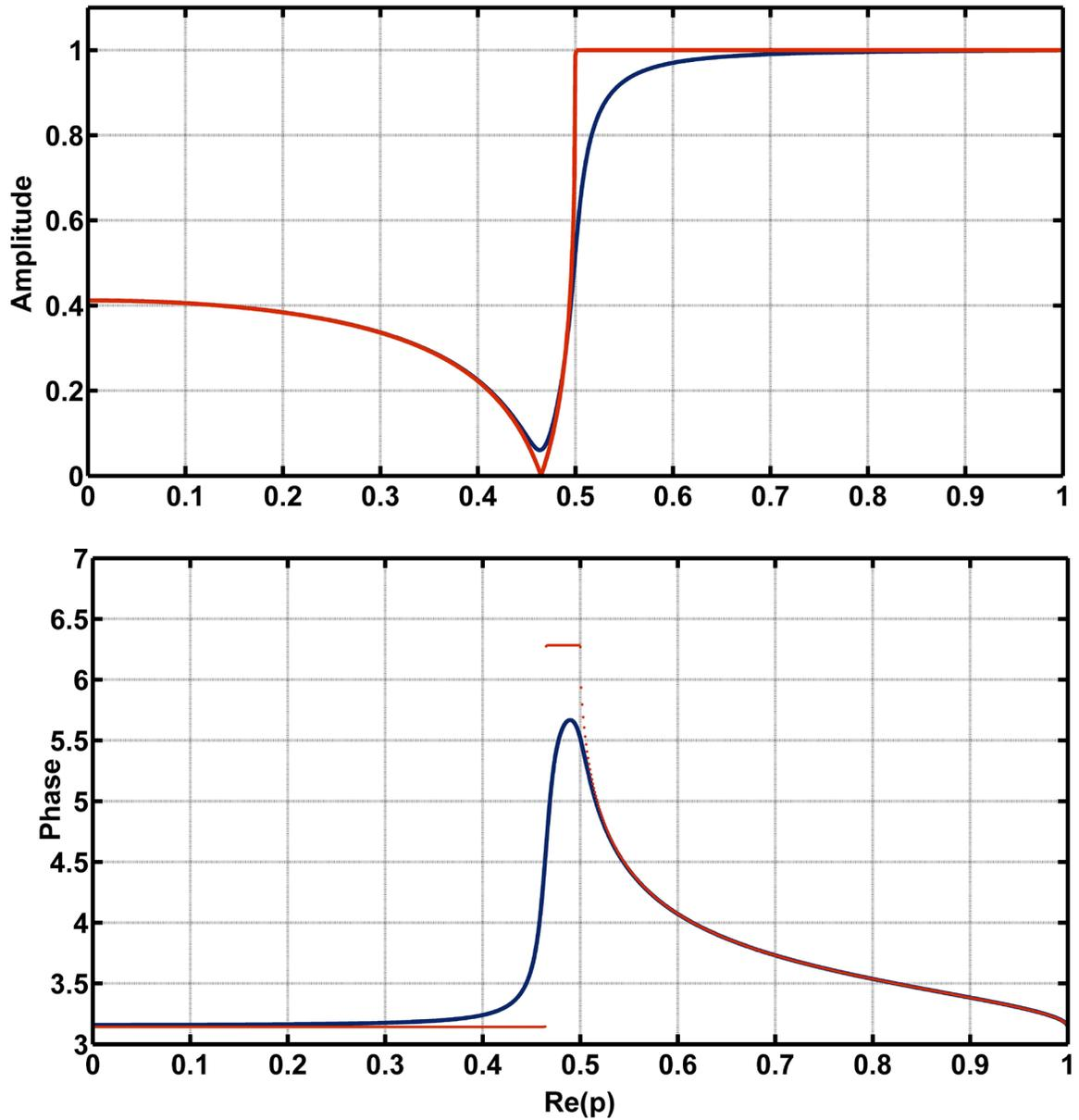
Fig. 2. The  $R_{11}^{SH}$  reflection coefficient at an interface between two medium. The upper (1) medium is elastic while the lower (2) medium is poroviscoelastic with  $Q_2 = 30$ . Medium parameters are given in Table 1.
