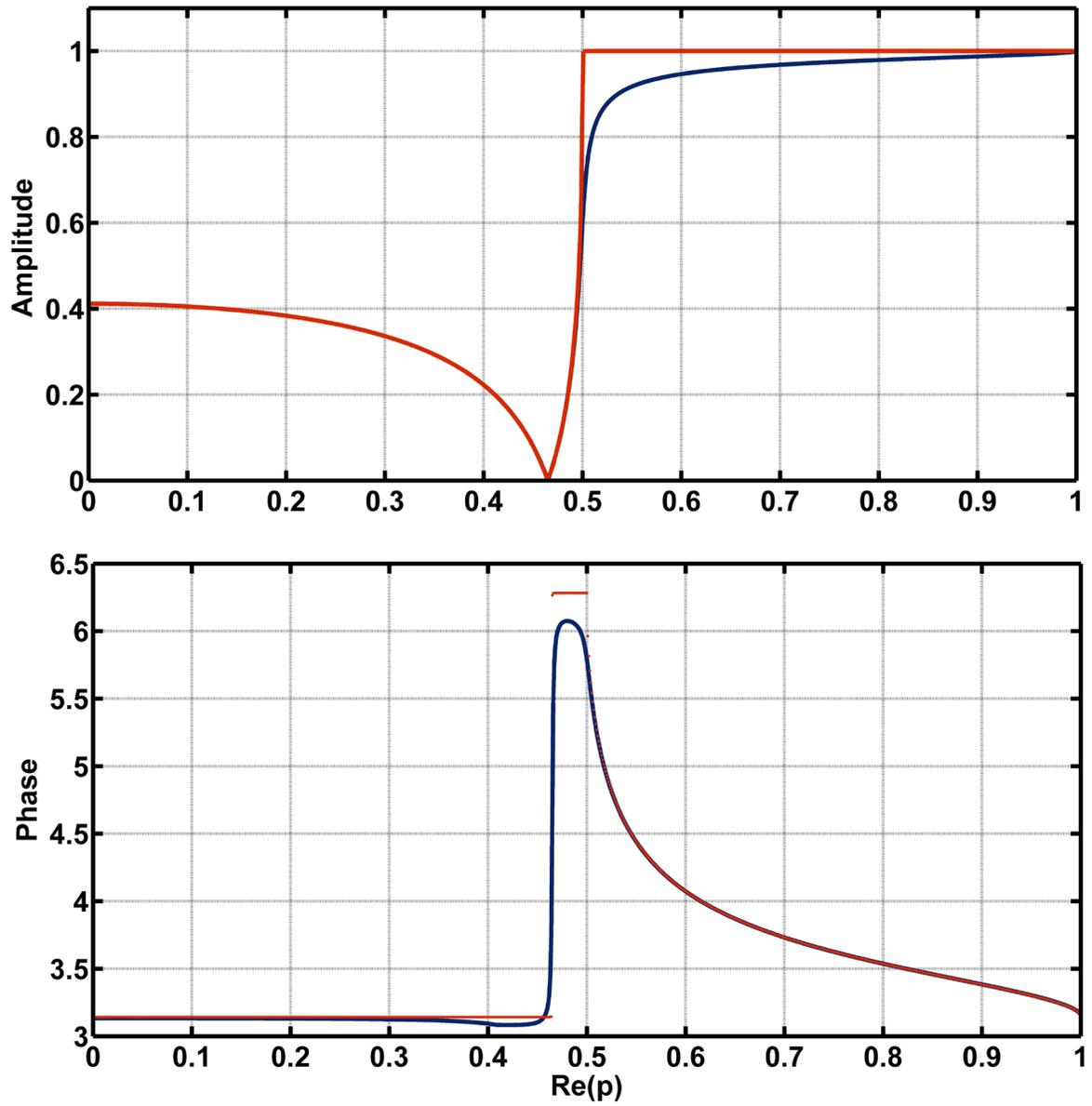
Fig. 8. The  $R_{11}^{SH}$  reflection coefficient at an interface between two medium. Both the upper (1) medium and the lower (2) media are anelastic with  $Q_1 = 20$  and  $Q_2 = 50$ . Medium parameters are given in Table 2.
