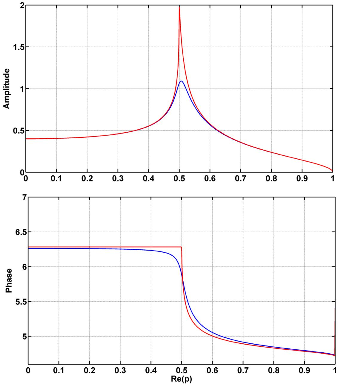
Fig. 4. The  $R_{12}^{SH}$  transmission coefficient at an interface between two medium. The upper (1) medium is elastic while the lower (2) medium is poroviscoelastic with  $Q_2 = 30$ . Medium parameters are given in Table 1.
