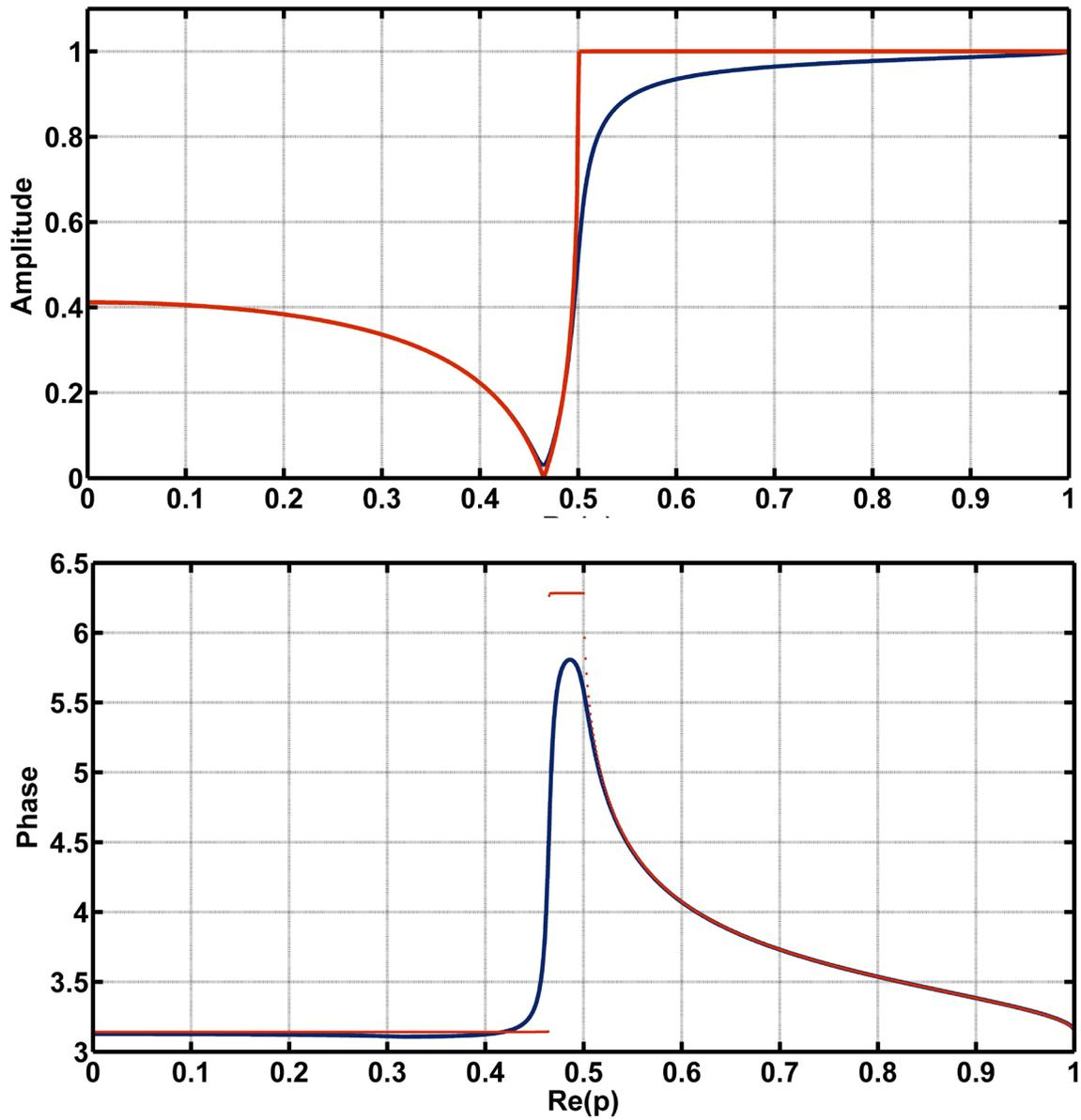
Fig. 9. The  $R_{11}^{SH}$  reflection coefficient at an interface between two medium. Both the upper (1) medium and the lower (2) media are anelastic with  $Q_1 = 20$  and  $Q_2 = 30$ . Medium parameters are given in Table 2.
