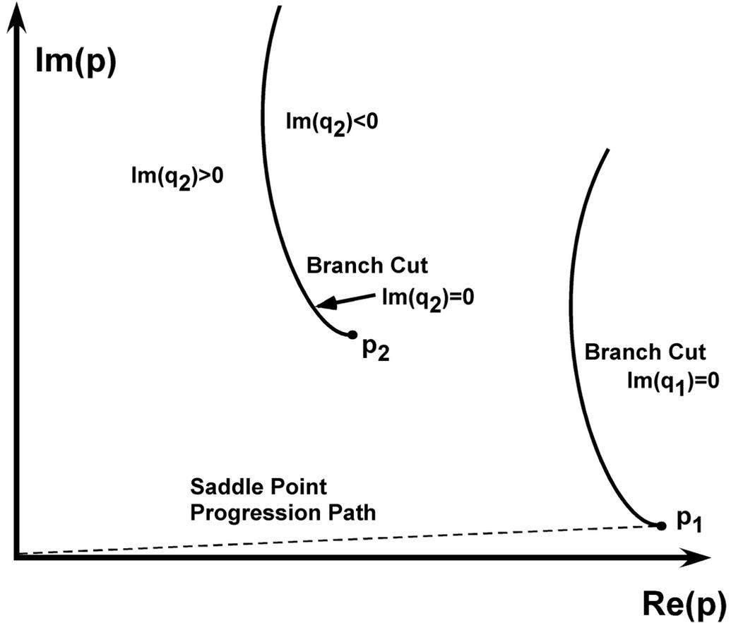
Fig. 1. This schematic shows the saddle point path for the zero – order saddle point approximation for the  $SH$  wave equation for shear wave reflection from the plane interface between the two media. The parameter values in Table 1 indicate that the saddle point path should lie along the real  $p$  – axis . It has been moved slightly into the first quadrant for viewing convenience.
