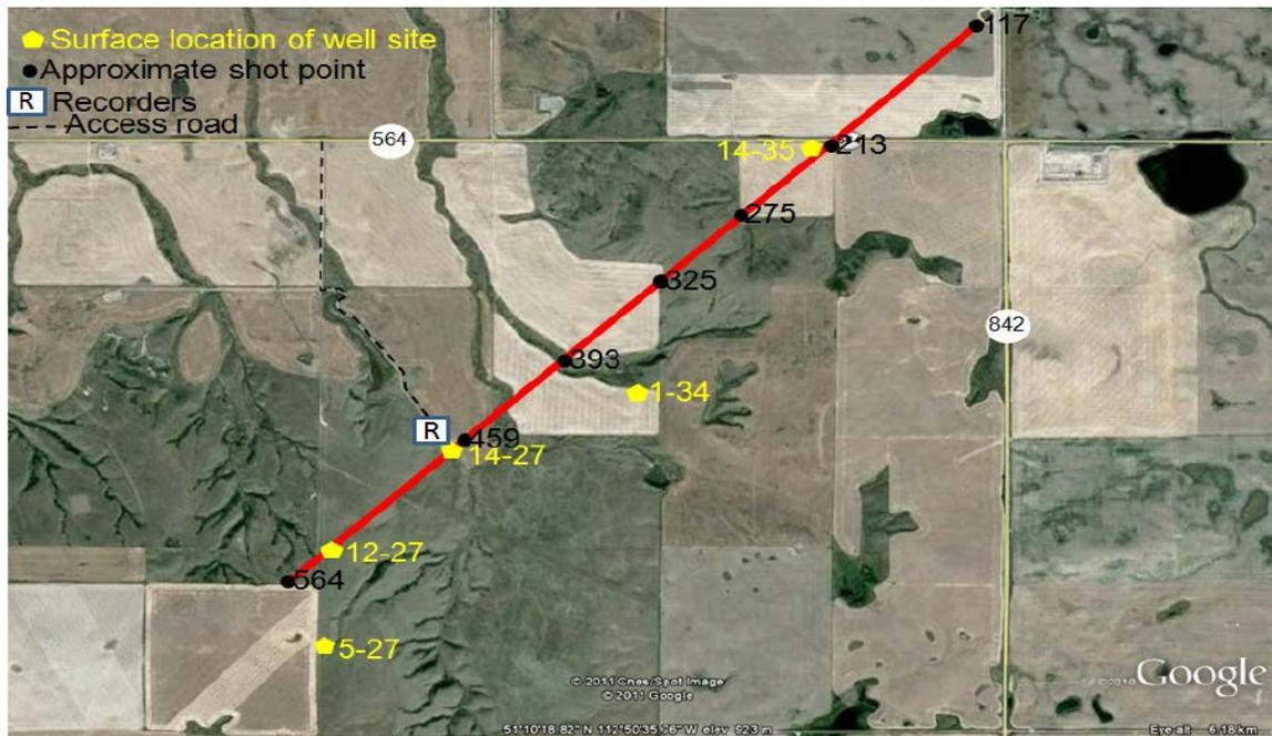
FIG. 1: Location of the Hussar seismic line with nearby wells, and shot locations. Well 12-27 provided dipole sonic logs; wells 14-27 and 14-35 only provided P-wave logs. (Margrave et al., 2011).
