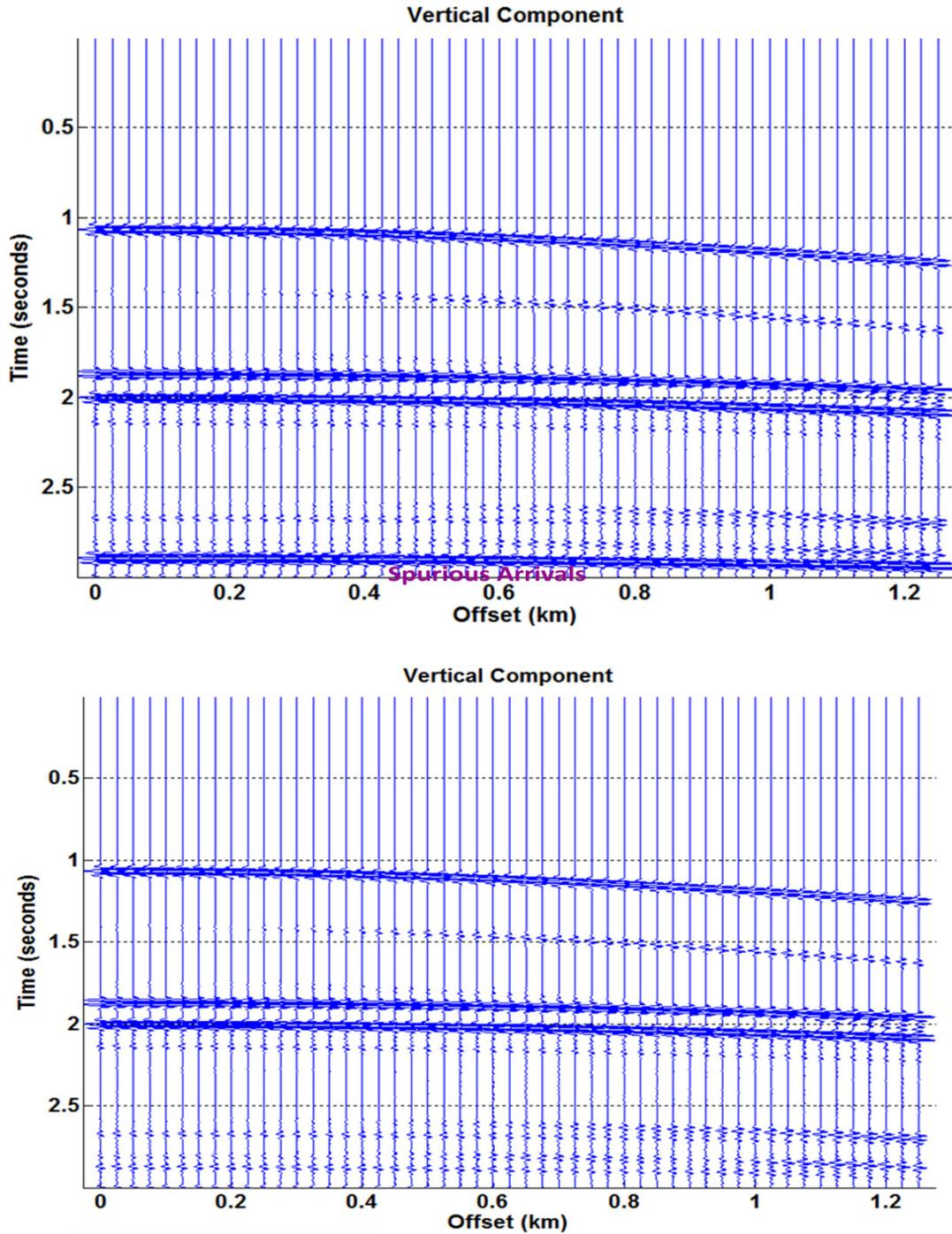
Fig. 4: The vertical component of the offset synthetic of the model described in the text. In the upper panel there are mild spurious reflections from the model bottom while in the lower panel these have been removed.
