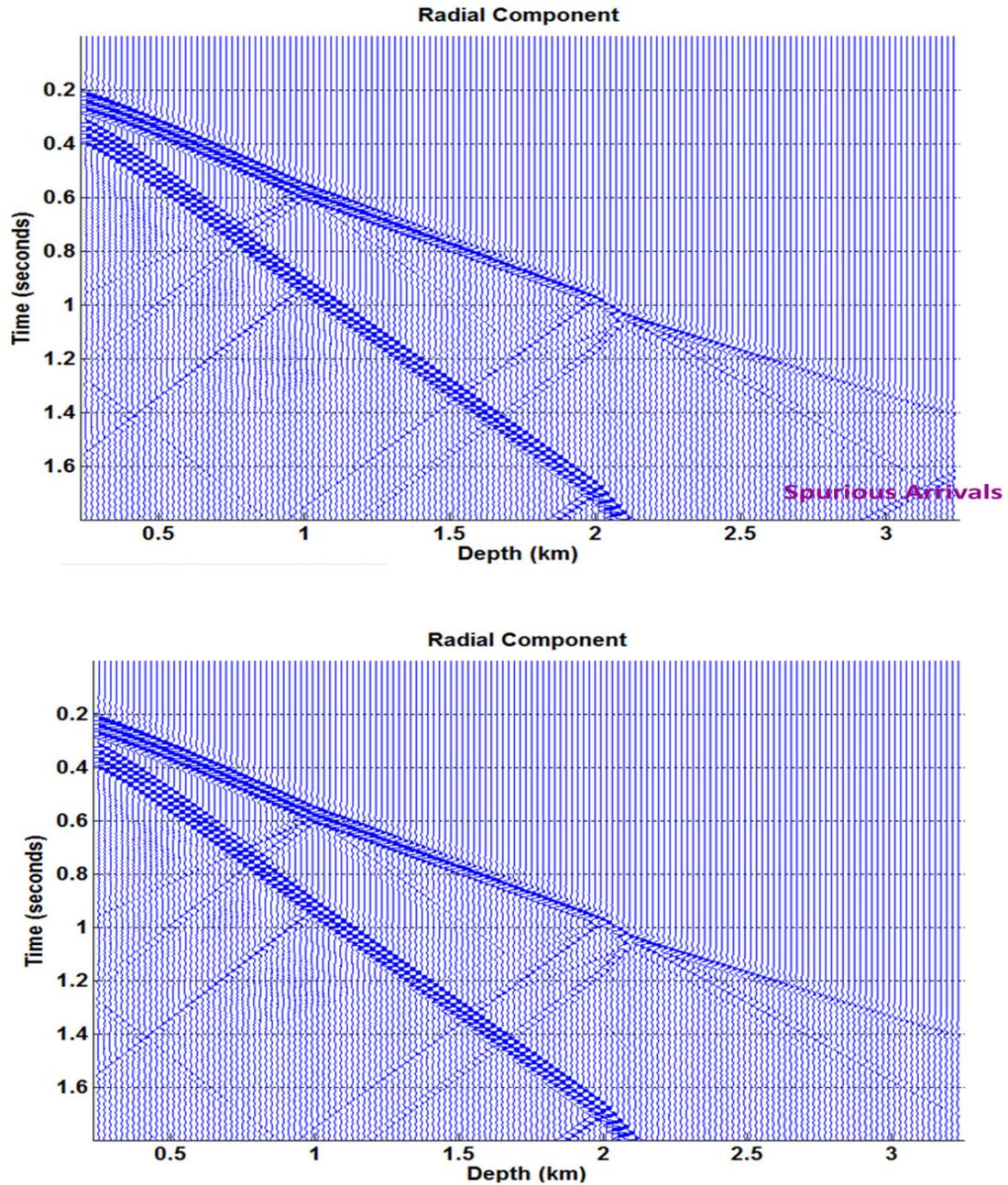
Fig. 3: The radial component of the VSP synthetic of the model described in the text. In this panel the computations continued to the proper time indicating that no spurious reflections from the model are included in the traces
