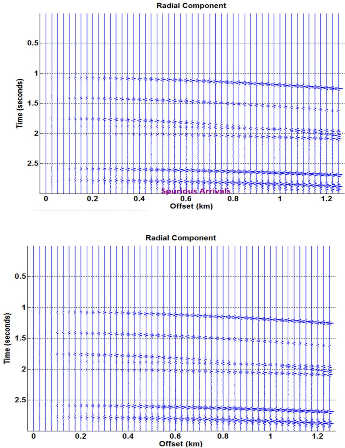
Fig. 5: The radial component of the offset synthetic of the model described in the text. In the upper panel there are mild spurious reflections from the model bottom while in the lower panel these have been removed.
