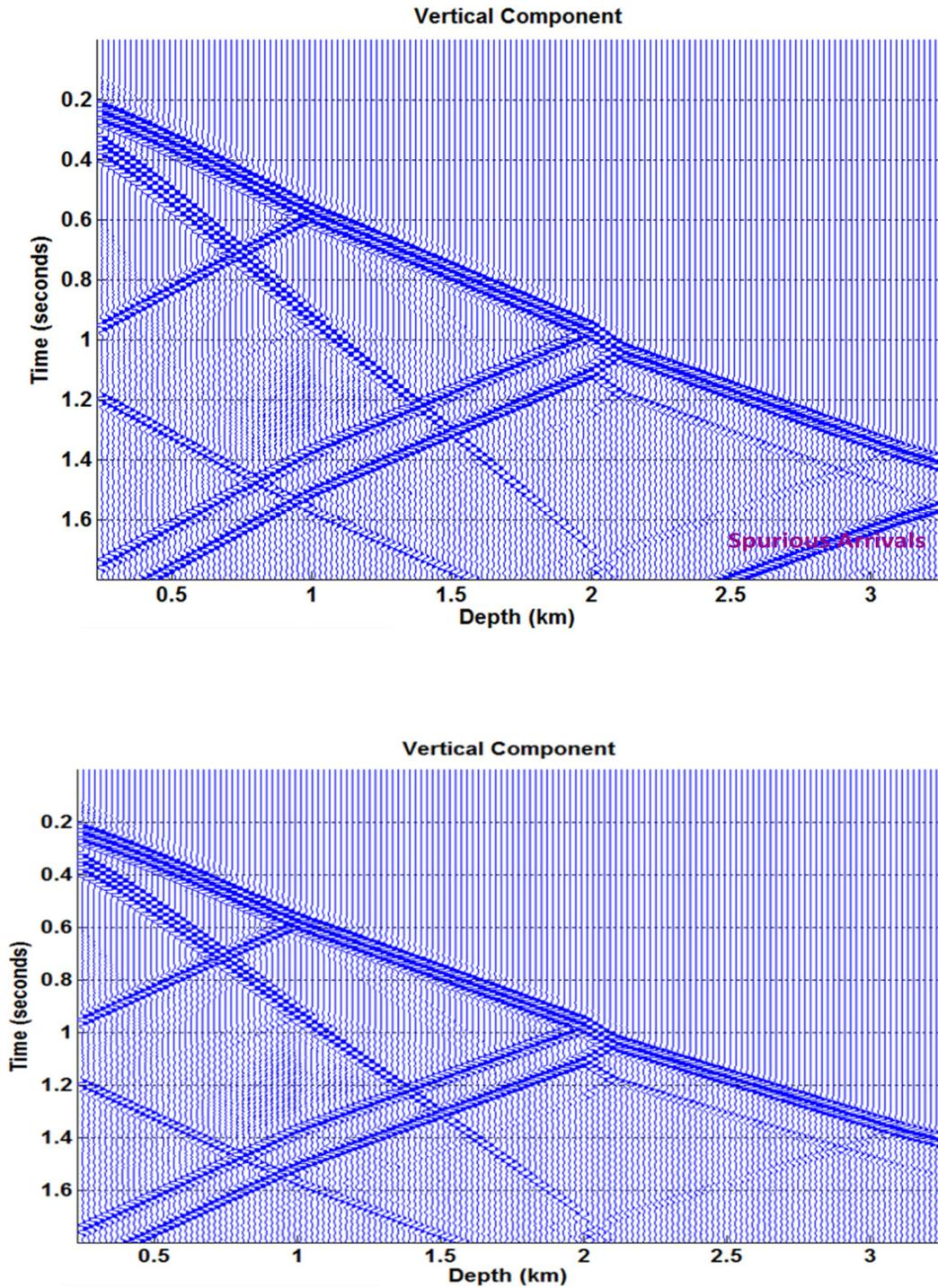
Fig. 2: The vertical component of the VSP synthetic of the model described in the text. In this panel the computations continued to the proper time indicating that no spurious reflections from the model are included in the traces.
