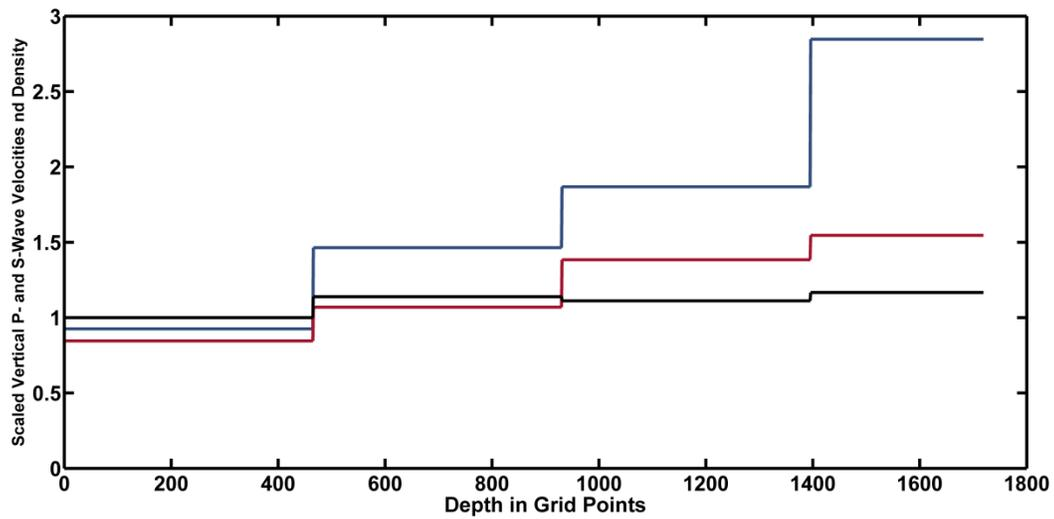
Fig. 6: The scaled vertical  $q_P$  and  $q_{S_v}$  velocities together with the density for the transversely isotropic medium used in the modeling of the next two figures.
