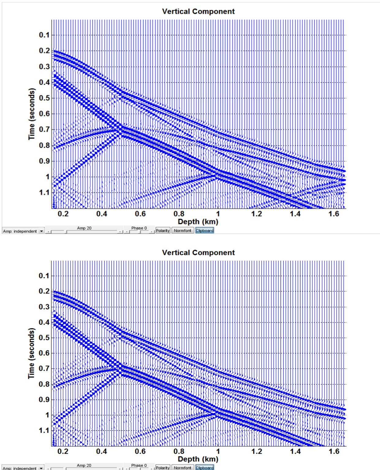
Fig. 7: The vertical component of the VSP synthetic for the model described in the text. In the upper panel the spurious reflections from the model bottom have not been removed. In the bottom panel they have. A comparison was done with a computationally intensive method and compared with almost no difference.
