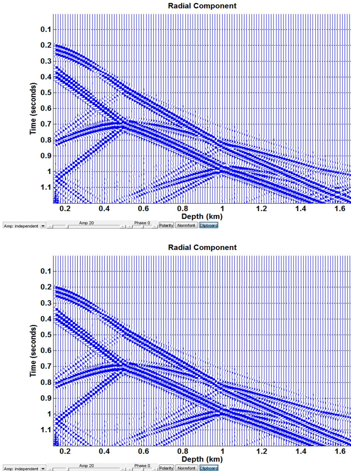
Fig. 8: The radial component of the VSP synthetic for the model described in the text. In the upper panel the spurious reflections from the model bottom have not been removed. In the bottom panel they have. A comparison was done with a computationally intensive method and compared with almost no difference.
