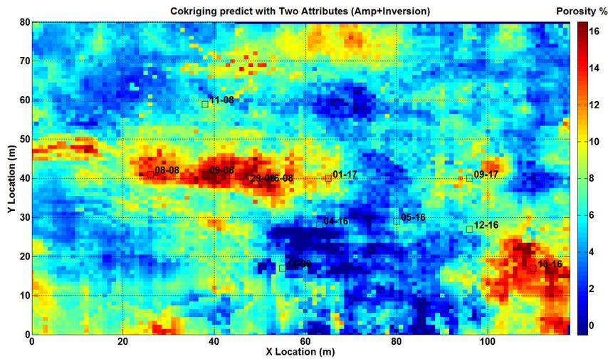
FIG. 9: Cokriging predict with two secondary data (inversion and seismic amplitude)
