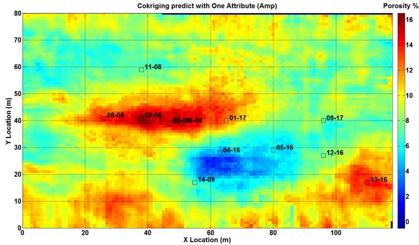
FIG. 8: Traditional cokriging prediction with seismic amplitude
