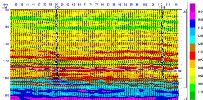
(b) P-wave impedance horizon slice
