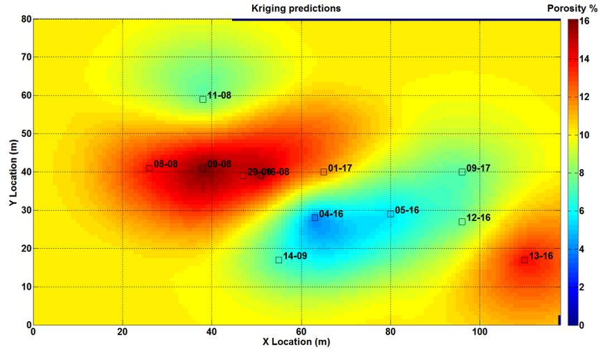
FIG. 6: Kriging interpolation with well log data
