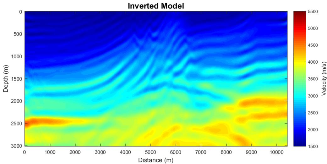
FIG. 6. Inverted model using the initial model on the top left of figure 3 and based on equation 26. The algorithm ran on a personal laptop without the need of parallel processing in about 36 hours.
