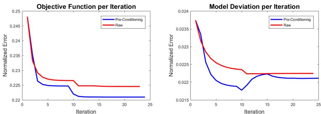
FIG. 10. Plots of the objective function per iteration (left) and model deviation per iteration (right) with the "raw" gradient (red) and pre-conditioned one (blue).
