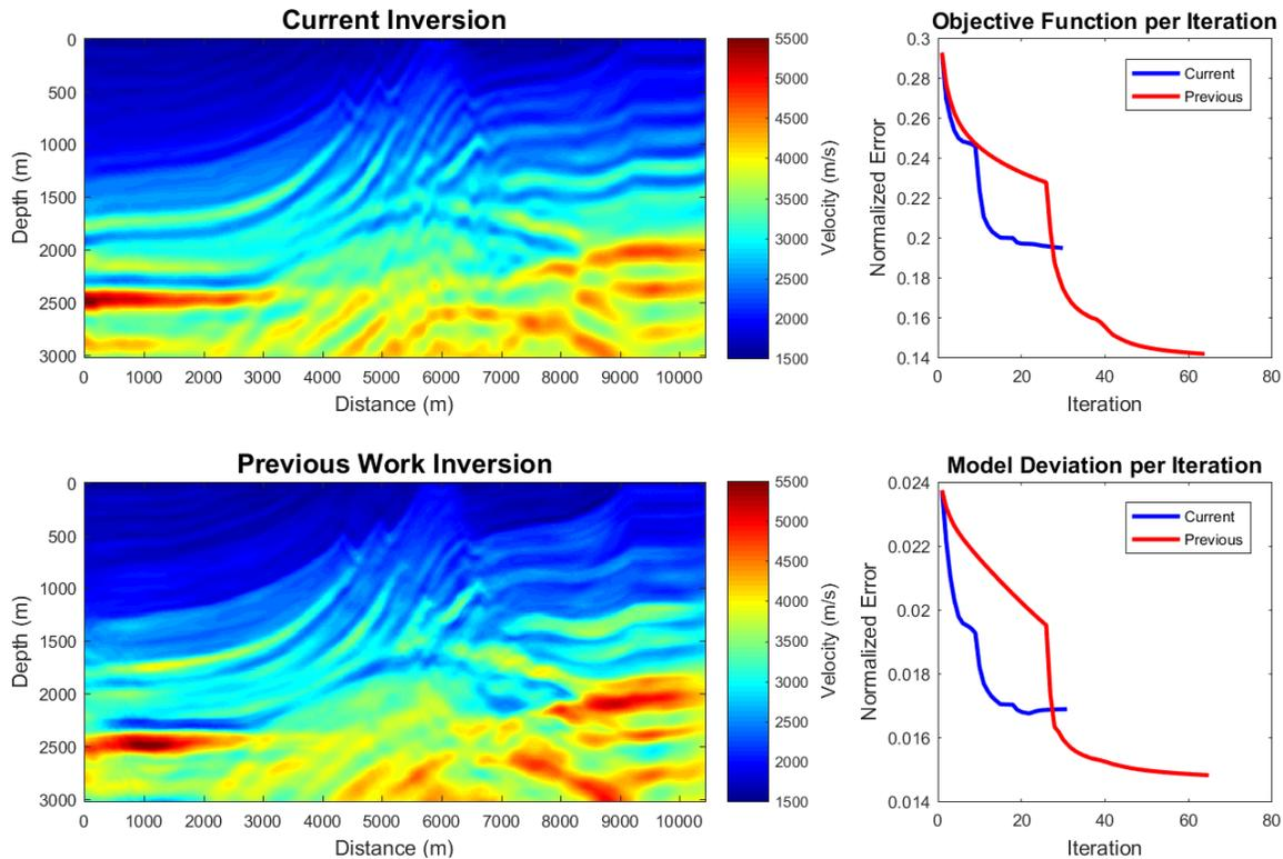
FIG. 5. On the left are the resulting velocity models on current (top) and previous (bottom) work inversions. On the right are the comparison of the objective function (top) and models deviations (bottom) per iteration.
