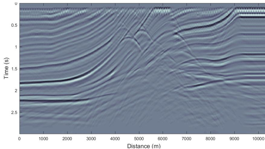
FIG. 8. Stacked section used as input in the post-stack method.
