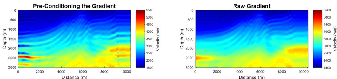
FIG. 9. Inverted models using: pre-conditioned gradient (left) and the "raw" one (right).
