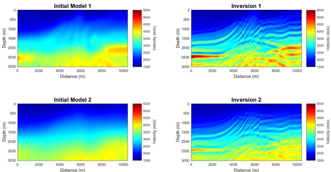
FIG. 3. Inversion as a function of the initial model. The inversion 1 has more details than the inversion 2 due to the initial model be closer to the local minimum.
