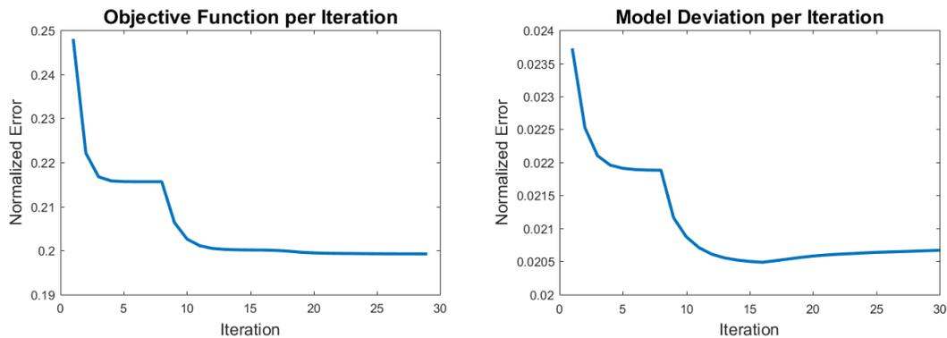
FIG. 7. Plots of the objective function per iteration (left) and model deviation per iteration (right). There was a total of 23 updates in the model but the convergence is reached with only 12.
