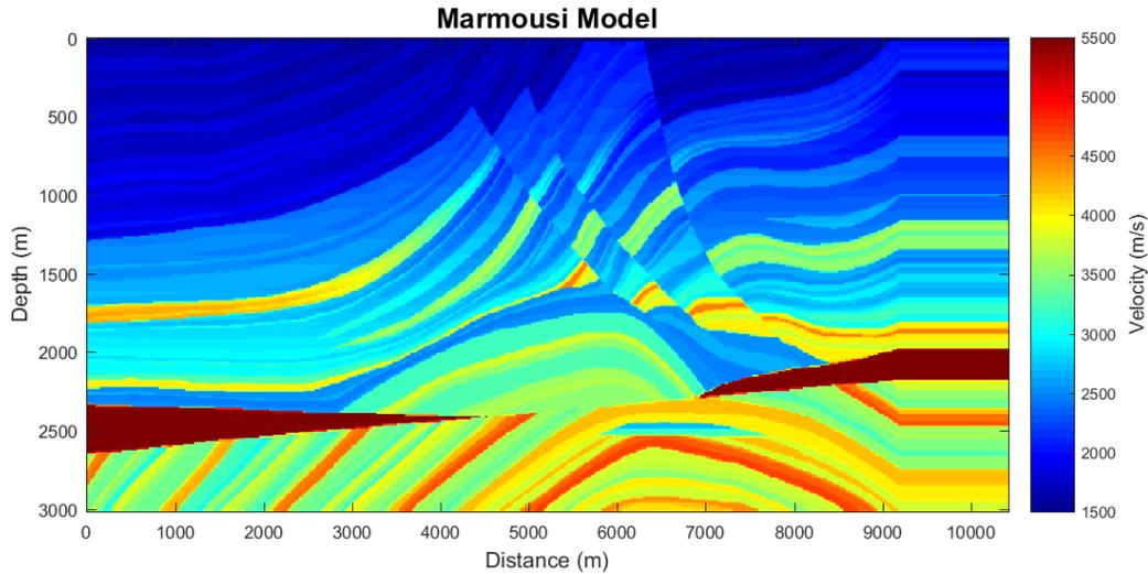
FIG. 1. The Marmousi 2D model. The color bar indicates the wave propagation velocity in m/s.
