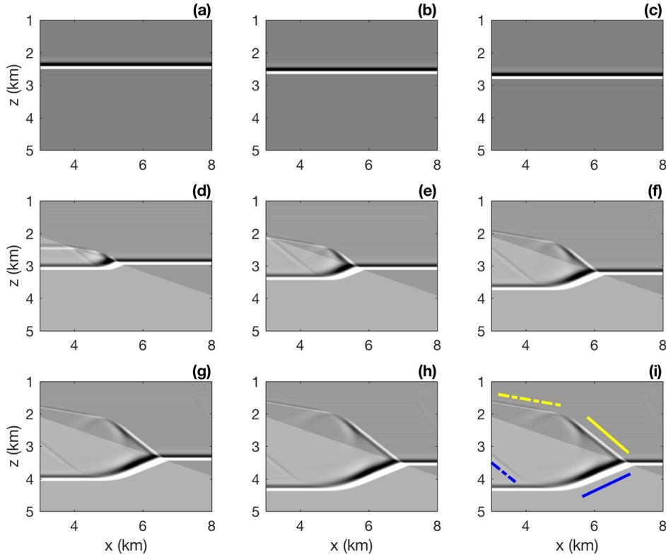
FIG. 7. Snapshots of wavefront interacting with a boundary involving both time- and space-boundary components.
