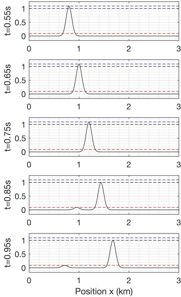
FIG. 1. Five snapshots of a waveform propagating through a 1D scalar acoustic medium, as computed with a simple finite difference solver. At  $t=0.75\text{s}$ , the velocity of the homogeneous medium is rapidly altered from  $2.0\text{km/s}$  to  $2.4\text{km/s}$ . The reference amplitude values of  $1.091$ ,  $1$ , and  $0.091$  are labelled with blue, black and red dashed lines respectively.
