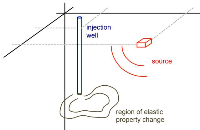
FIG. 10. Scheme: a reservoir setting in which (perhaps by a rapid pressuring-up) medium properties vary at the same time that they are illuminated by a seismic wave.
