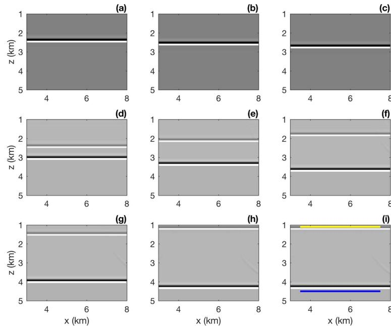
FIG. 6. Snapshots of wavefront interacting with a time-boundary at normal incidence.
