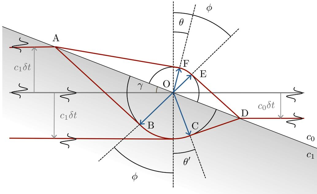
FIG. 9. Schematic representation of the wavefronts generated in the moments after a downward, vertically propagating wavefront has encountered a boundary with both time- and space- aspects.
