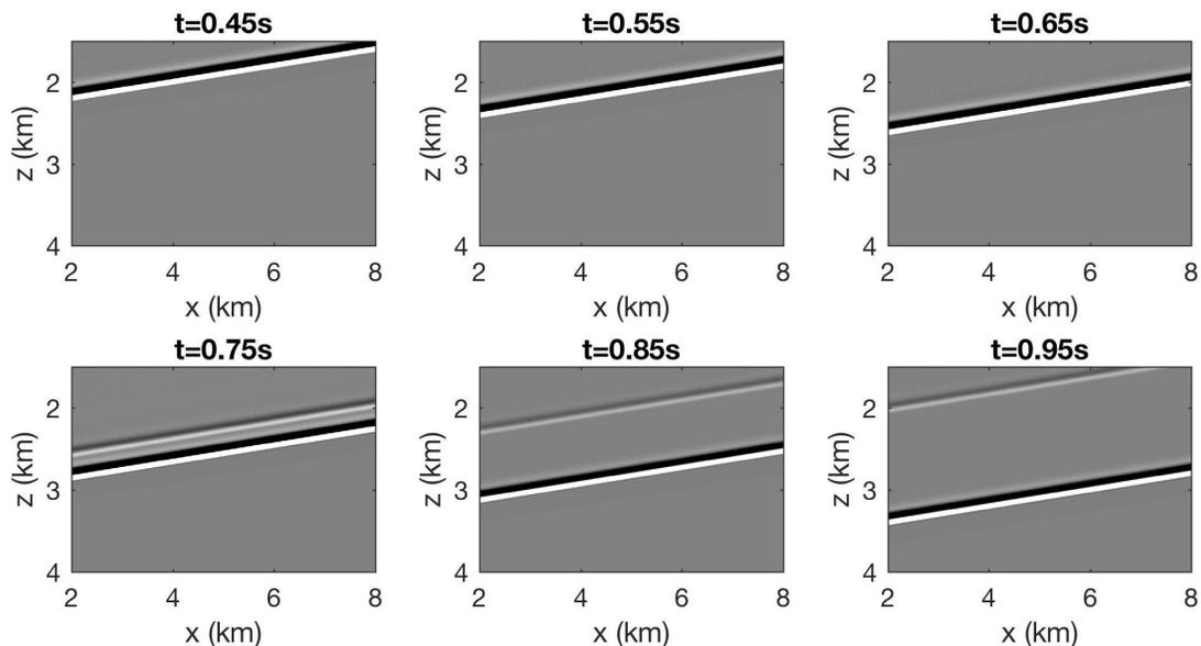
FIG. 2. A plane wave before and after its interaction with a time-boundary (occurring at 0.7s). Because the two emerging waveforms propagate forwards and backwards along the same propagation axis
