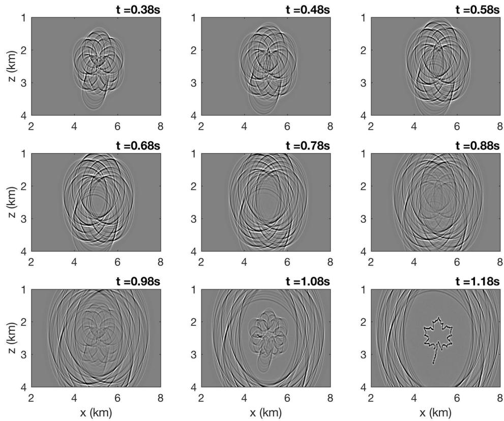
FIG. 3. Snapshots of a waveform on a (say) pond surface excited by a falling maple leaf. At 0.7s, caused by some unknown process, the surface wave velocity suddenly changes. The time-boundary reflected waveform re-focuses on the original source at 1.18s.
