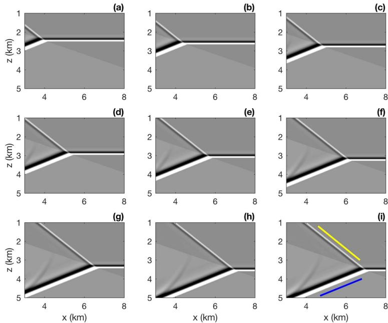
FIG. 5. Snapshots of wavefront interacting with a space-boundary at oblique incidence.
