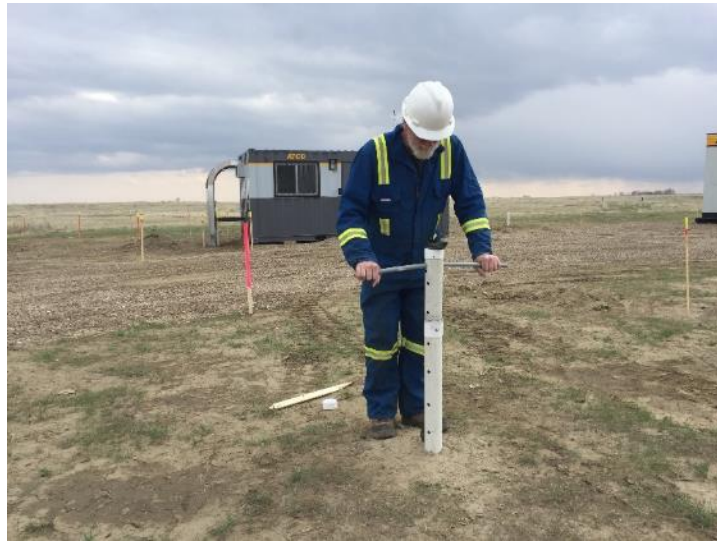
FIG 5. Malcolm Bertram orienting 3C geophone during installation.
