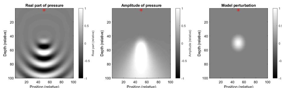
FIG. 1: Left: Real part of frequency domain radiation pattern. Center: Amplitude of frequency domain radiation pattern. Right: Variables considered in inversion. The red stars mark the source location. Changes in variables like this introduce limited reflections, allowing for the RWI strategy to be used without demigration. This should also allow for the natural treatment of diving waves simultaneously.
