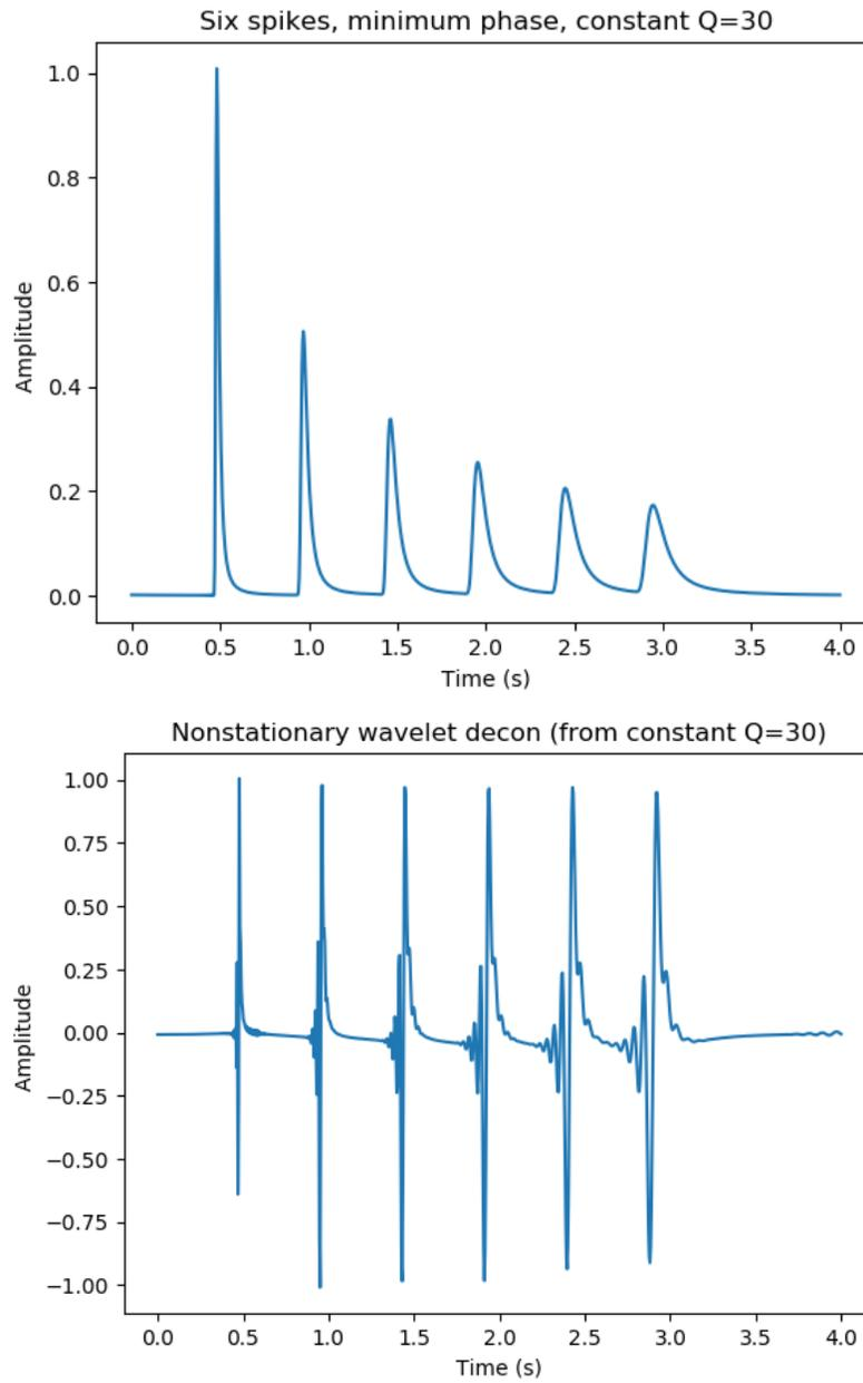
FIG. 4. Six spikes in a constant Q medium and the result of nonstationary wavelet deconvolution.
