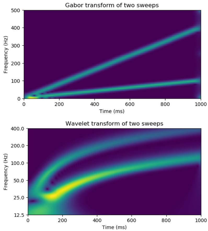
FIG. 3. Comparison of Gabor and Wavelet transforms. Note the resolution at low frequencies.
