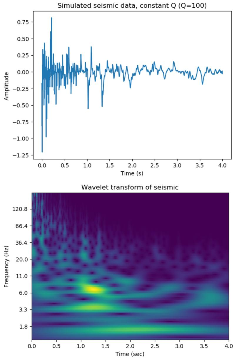
FIG. 6. Simulated constant Q seismic data, and CWT. Note the energy decay in higher frequencies.
