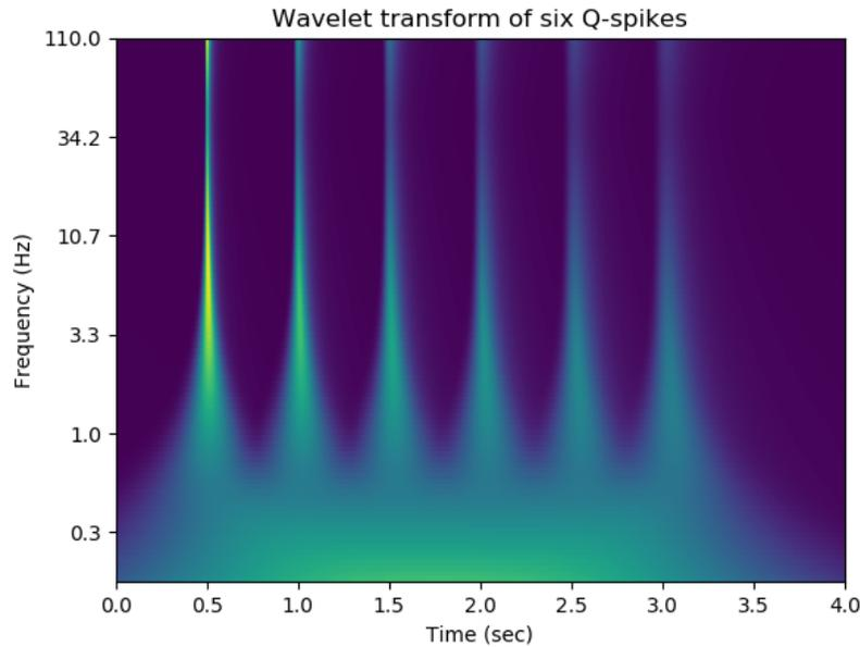
FIG. 5. For reference, the CWT of the six spikes in constant Q medium.
