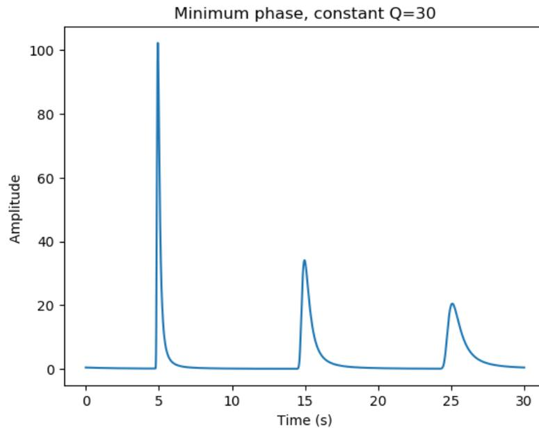
FIG. 1. Minimum phase impulses with constant Q attenuation.
