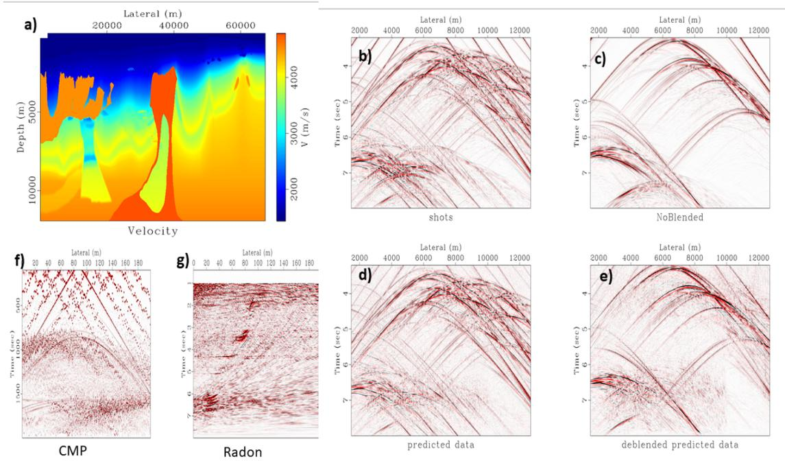
FIG. 9. Deblending by inversion in complex salt structure recording
