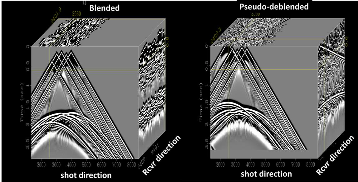
FIG. 4. Volume expansion produced by pseudo-deblending.
