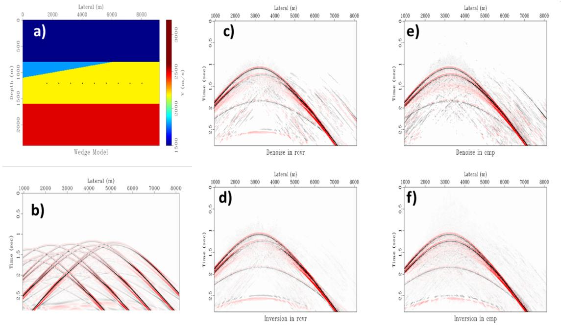
FIG. 8. Pushing the algorithms to the break-point: Deblending by denoising and inversion in CMPs and Receiver gathers for diffractions under a wedge.
