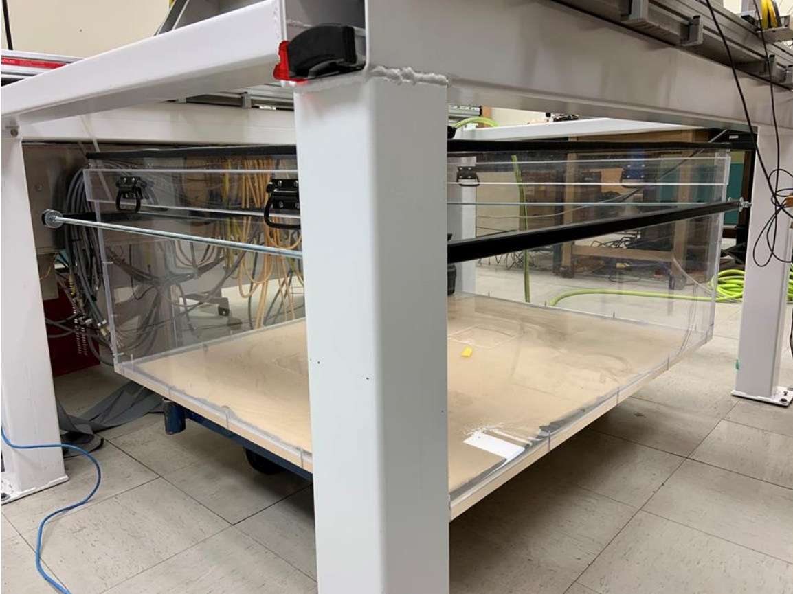
Fig. 2.1: Acrylic water tank. Note the black square steel tubing along the right side of the tank. A similar tubing runs along the opposite side. The two square tubings are held together by threaded steel rods at the front and back ends (the front rod is visible). The two square tubings are clamped tight against the tank sides with nuts and washers on the ends of the rods to prevent excessive bowing of the tank sides under water pressure.
