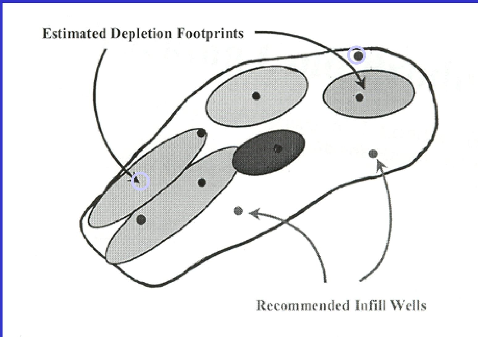
**Drainage footprint scenario for the cold production wells in a small southwest Saskatchewan heavy oil pool (Sawatzky, 2002)**
