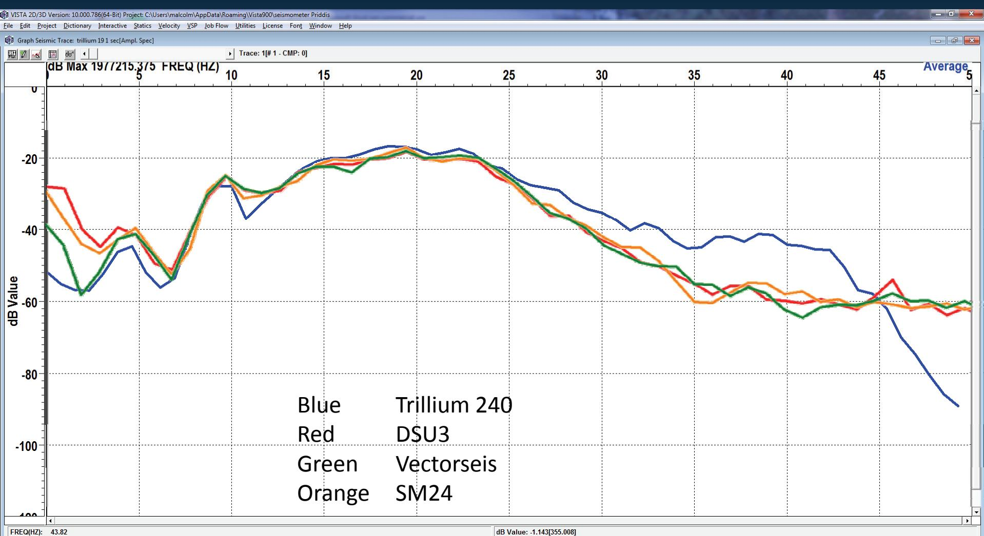
Geophone data convolved, MEMS data integrated, Seismometer data untouched
