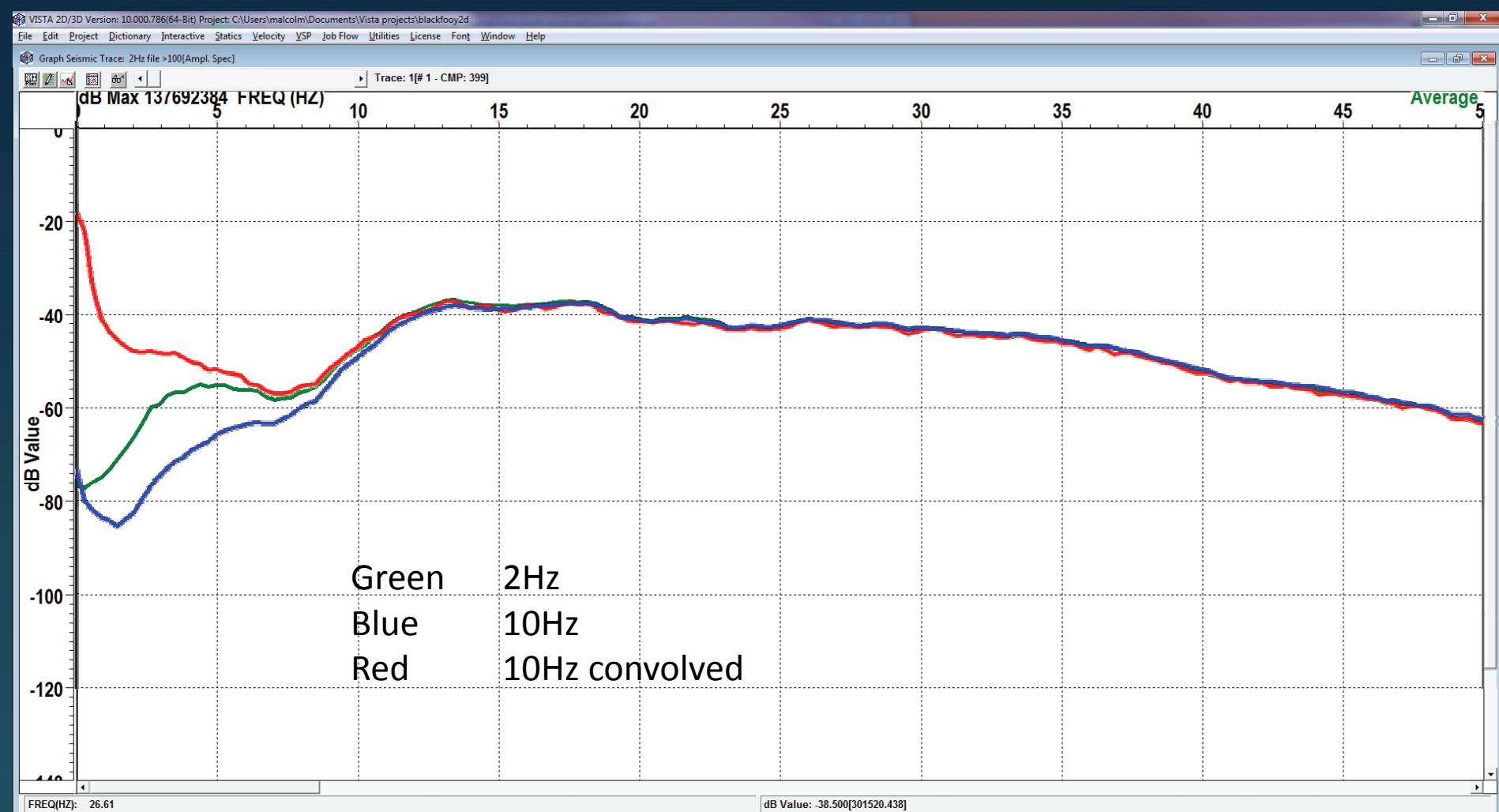
Average amplitude spectra 0-50Hz for offsets >100m
