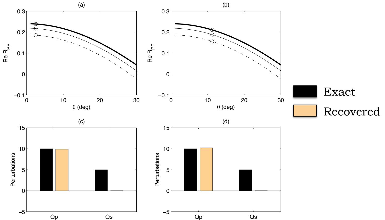
From  $R_{\text{PP}}$  AVF: target  $Q_p$  recovered,  $Q_s$  not
