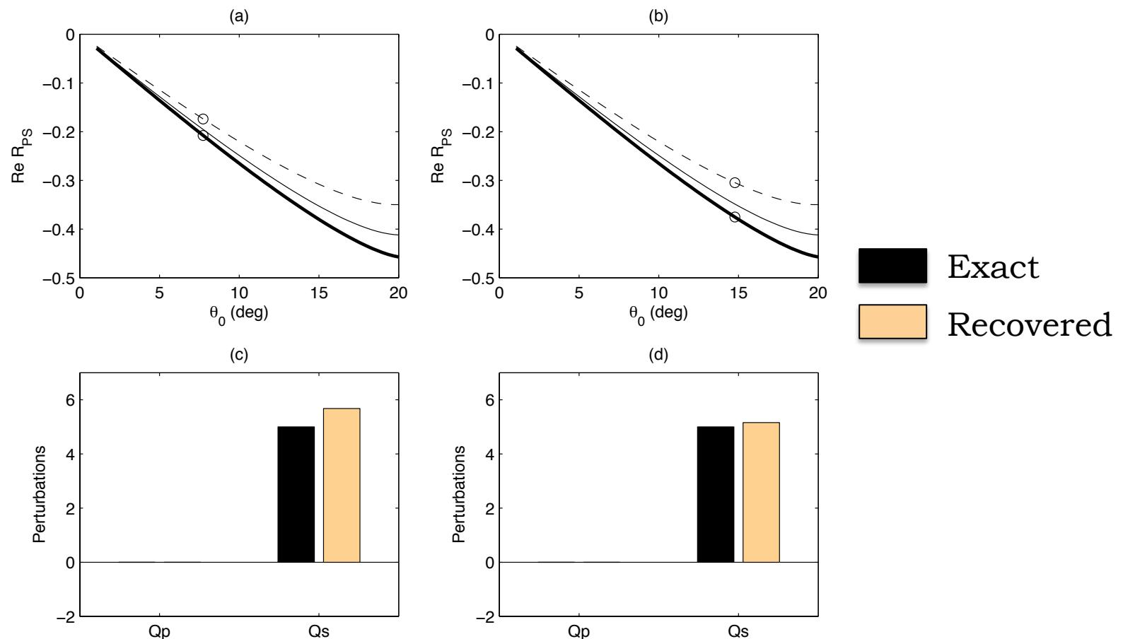
From  $R_{\text{PS}}$  AVF: target  $Q_s$  recovered,  $Q_p$  not
