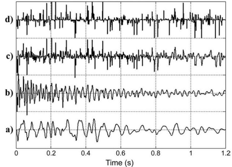
Q varies in time and frequency (left side above) (from Margrave et al., 2011). Georadargram (a, right side) is low resolution compared with the ideal (d). Gabor deconvolution (c) is superior to conventional deconvolution (b).
