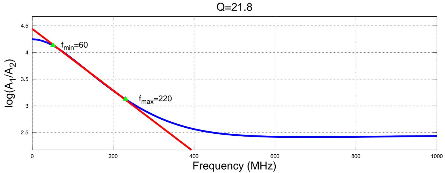
$Q$  estimation by the spectral-ratio method.
