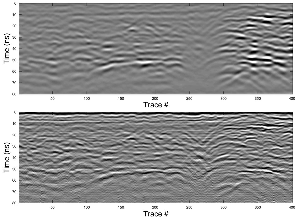
An earthquake fault in Italy. Conventional processing (top). Gabor deconvolution (bottom).
