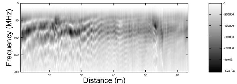
The bandwidth of the **raw data** is 20 - 200 MHz, and  $f_{dom} \sim 75$  MHz.
