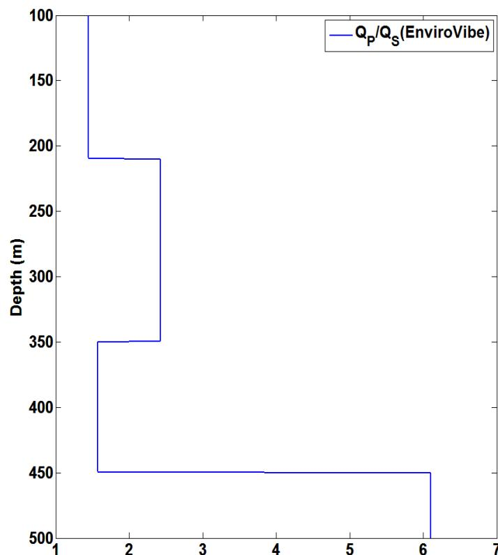
Spectral-ratio method from VISTA software
