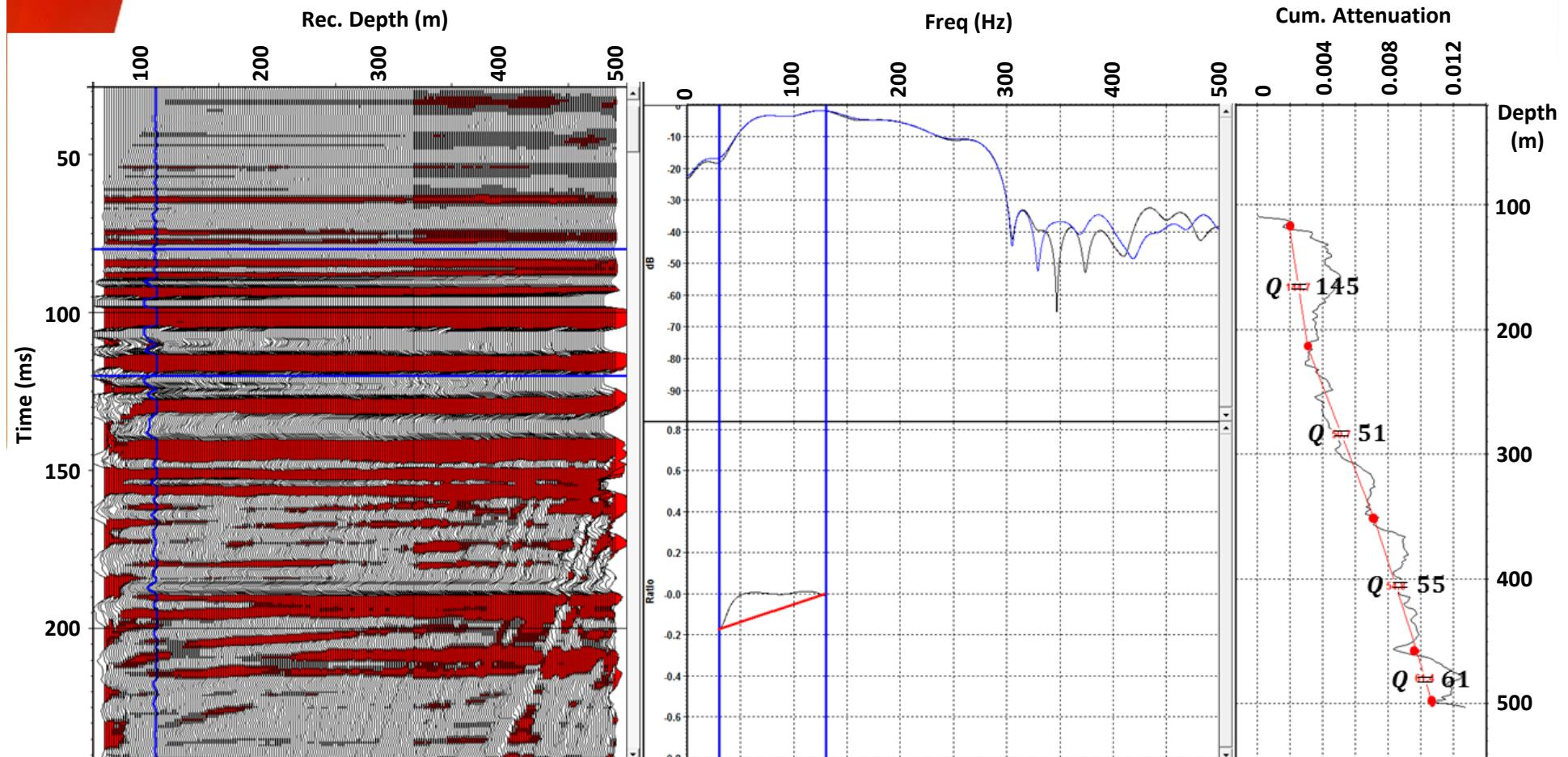
Spectral-ratio method from VISTA software.
