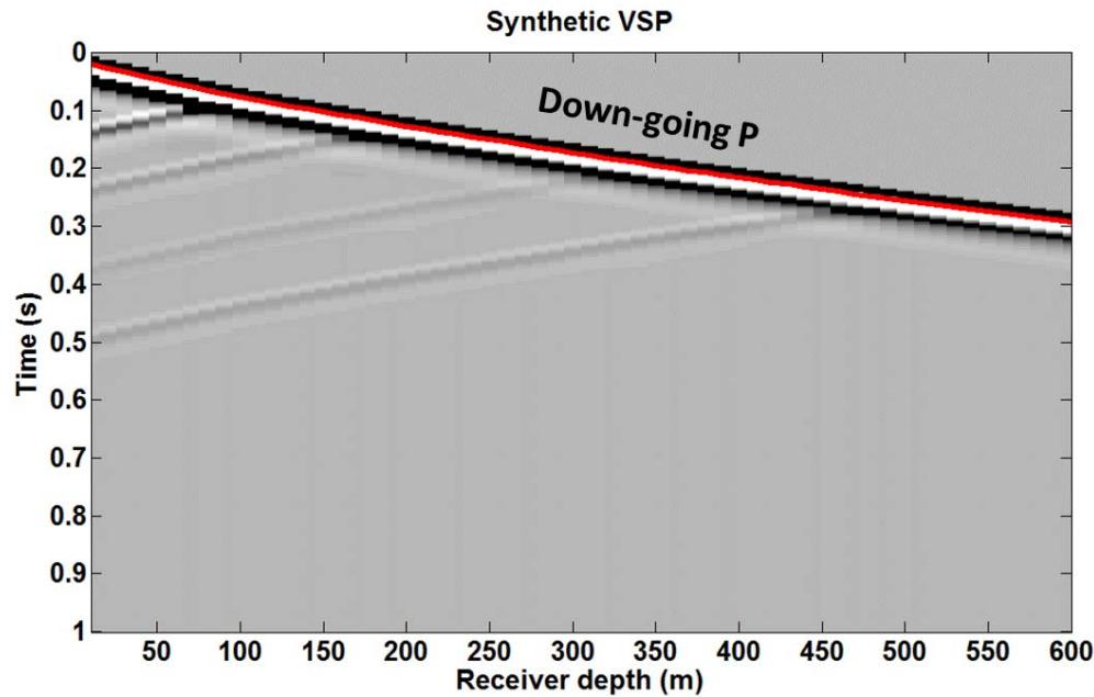
Diagram for  $Q_P$  estimation from synthetic down-going wavefield using the dominant frequency method from CREWES toolbox
