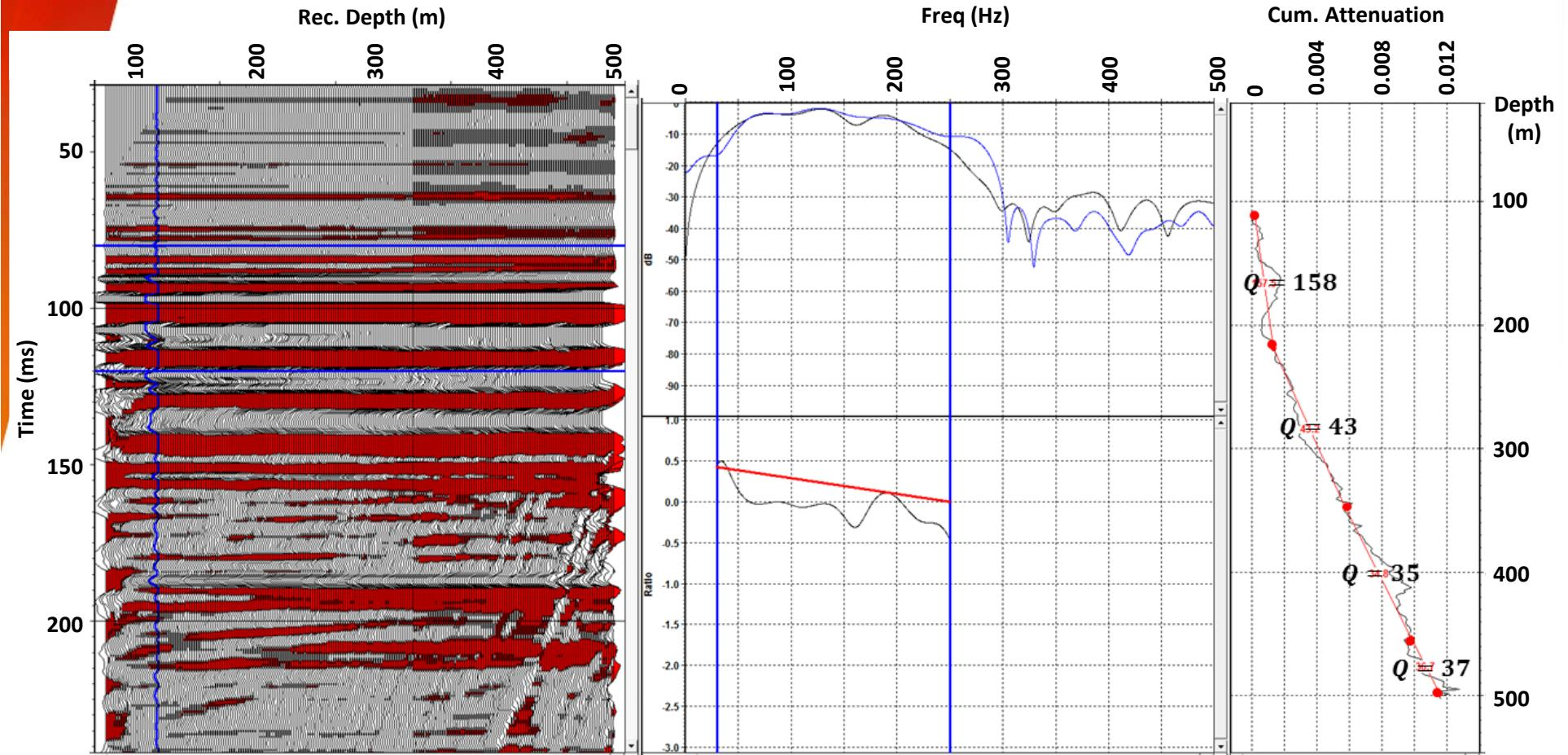
Spectral-ratio method from VISTA software.
