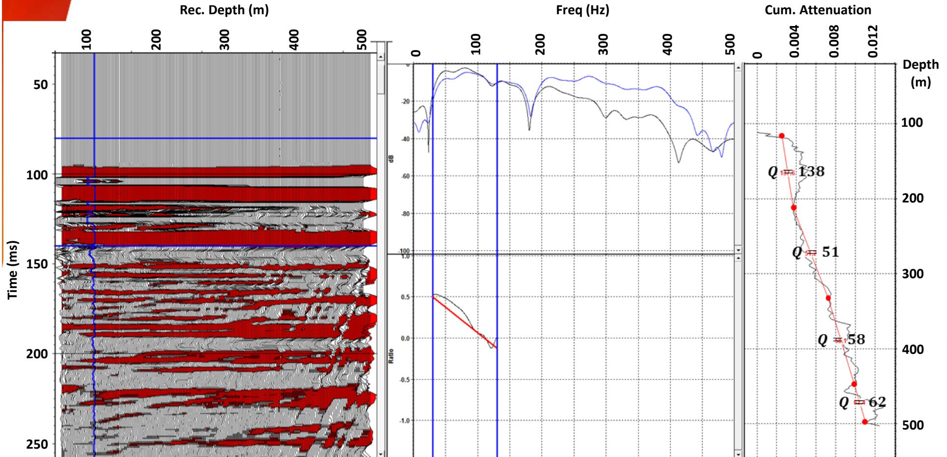
Spectral-ratio method from VISTA software
