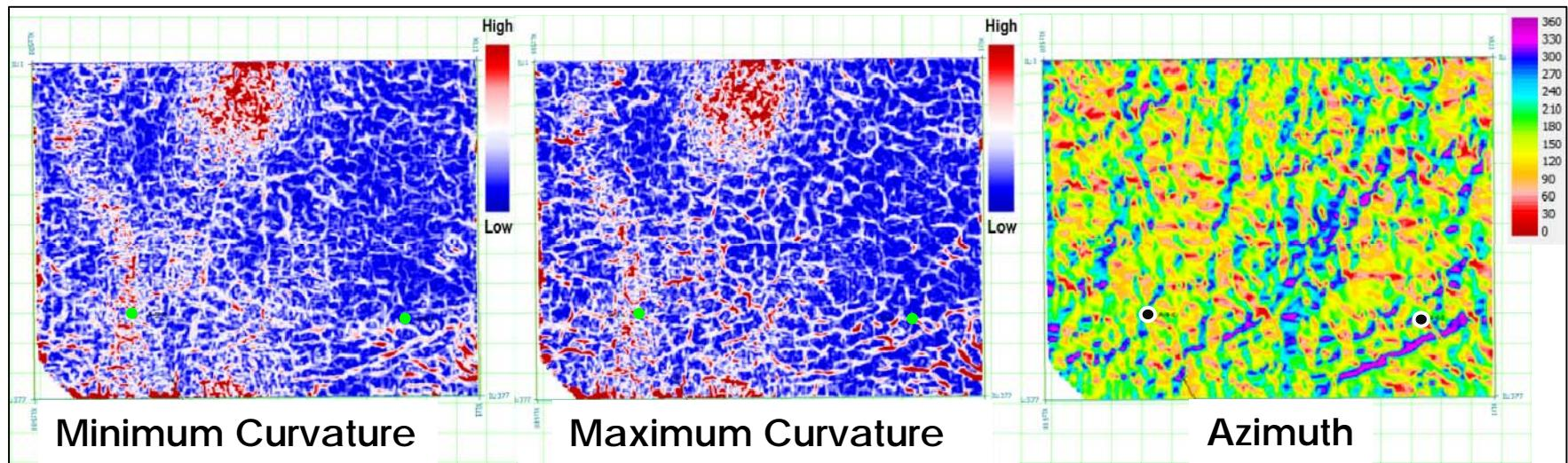
High curvature values indicate fractured zones. Azimuth map indicates that the major trends are about  $0^\circ$  and  $40^\circ$ .
