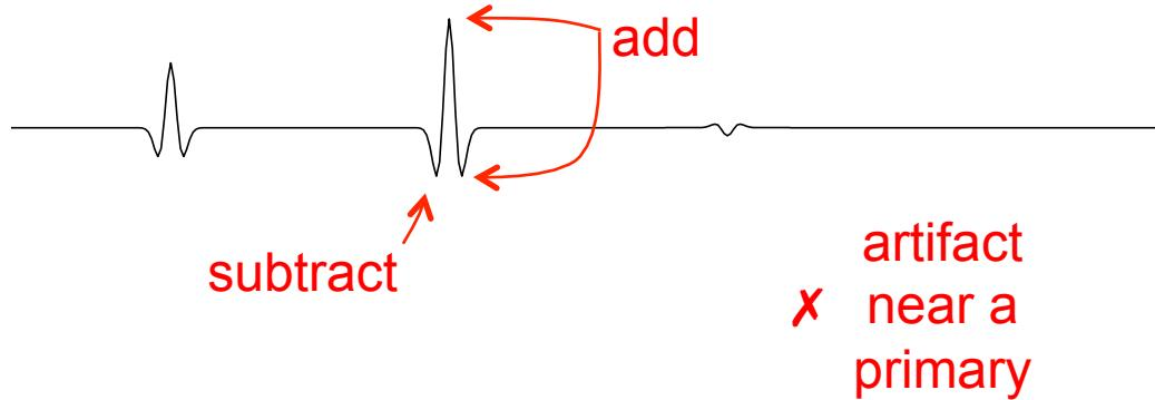
$$t_{\text{im}} = t_{p1} + t_{p2} - t_{p3}$$
