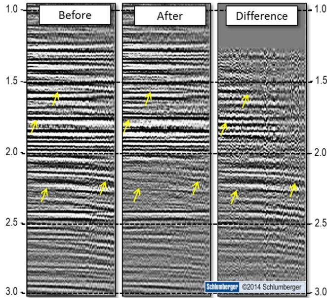
Figure 3 – CMP gathers before and after ISS multiple attenuation. Arrows indicate where strong multiples were removed. Gather difference shows strong multiples that were attenuated.
