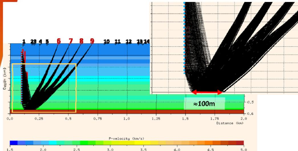
Ray-tracing for shot points 6 – 9 using NORSAR2D software
