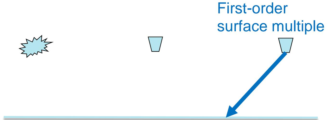
Fig 1. Forward and backward wave propagation in RTM with surface multiple
