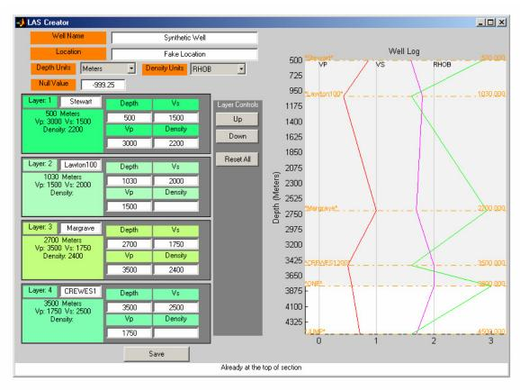
FIG. 4. The GUI for the lascreator program.
