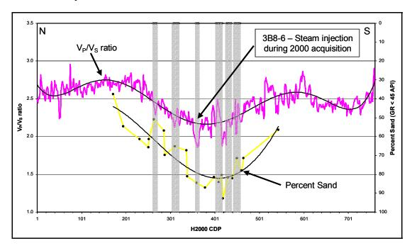
Fig. 10. Comparison of  $V_P/V_S$  trend line (left axis) with percent sand (reversed right axis) in the wells along H2000 (converted wave) (modified after Watson et al., 2002)
