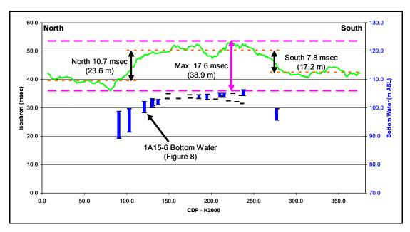
Fig. 7. Chart of the isochron thickness of the Prairie Evaporite (left axis) and the structural position of bottom water in the Waseca reservoir in the wells along H2000 (right axis)
