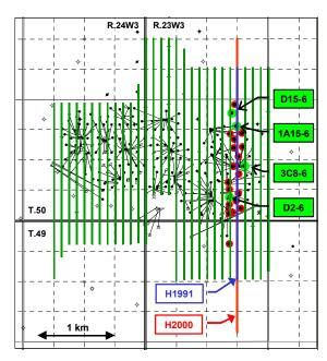
Fig. 1. Map of Pikes Peak field with wells and seismic coverage. 24 highlighted wells project 110 m or less on to the time-lapse seismic lines, H1991 and H2000.
