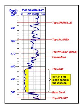
Fig. 11. Gamma ray log from well 3B9-6 indicating 57% sand (or 18 m) within the Waseca interval using a 45° API cut-off.
