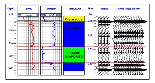
Fig. 5. Synthetic (normal polarity) tie from well 10-09 to H2000 over the Devonian section.
