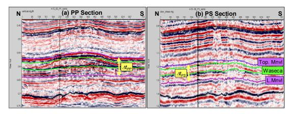
Fig. 9. Interpreted (a) PP (vertical component) and (b) PS (radial component) H2000 sections. Note the different time scales (modified after Watson et al., 2002).
