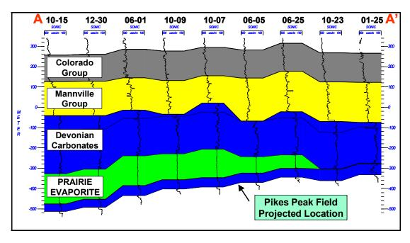
Fig. 4. Structural cross-section A-A' created with sonic logs (modified after Van Hulten, 1984). Note how the thickness of the Prairie Evaporite varies from 150 to 0 m (west to east) counter to regional dip (east to west).
