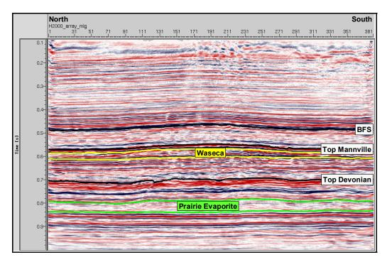
Fig. 6. H2000 (vertical array) seismic line with an interpretation of the top and base of the Prairie Evaporite and other major horizons.
