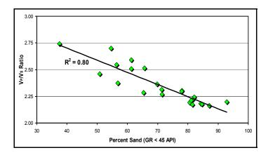
Fig. 12. Cross plot of V<sub>P</sub>/V<sub>S</sub> trend line versus percent Waseca sand in 23 wells along H2000
