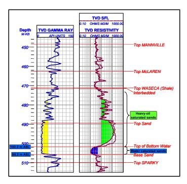
Fig. 8. Gamma ray and resistivity logs from sample well, 1A15-6, over the upper Mannville. 4 m of bottom water is present at the base of the Waseca sands.
